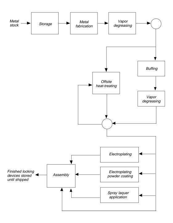
Figure 1. Abbreviated process flow diagram for locking device fabrication.
