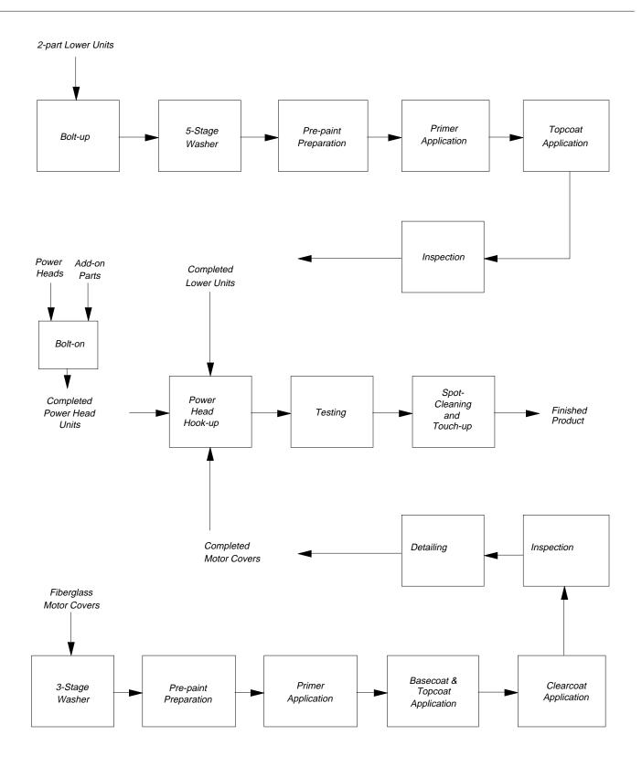
Figure 1. Abbreviated process flow diagram for outboard motor production.
