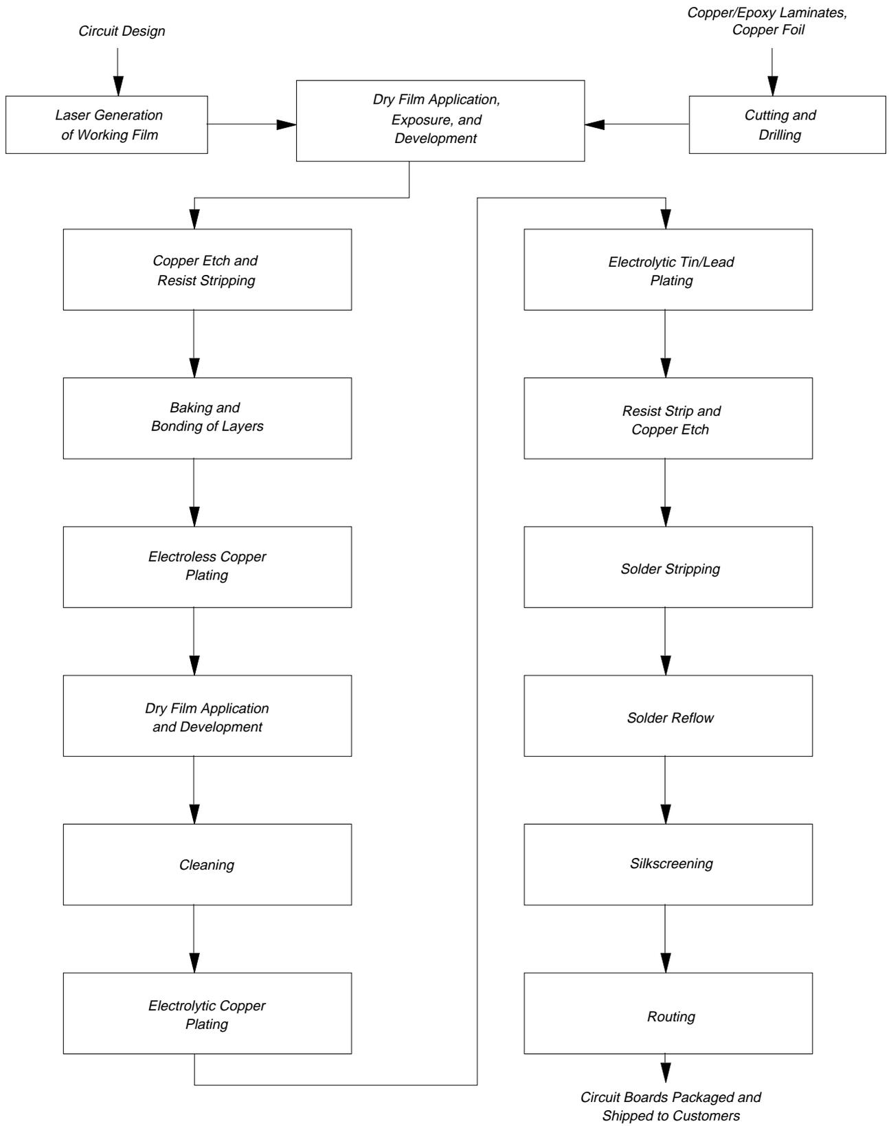
**Figure1.** Abbreviated process flow diagram for circuit board production.
