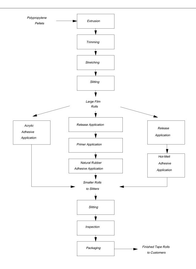
Figure 1. Abbreviated process flow diagram for pressure-sensitive adhesive tape production.
