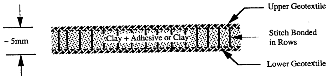
(b) Stitch Bonded Clay Between Upper and Lower Geotextiles
