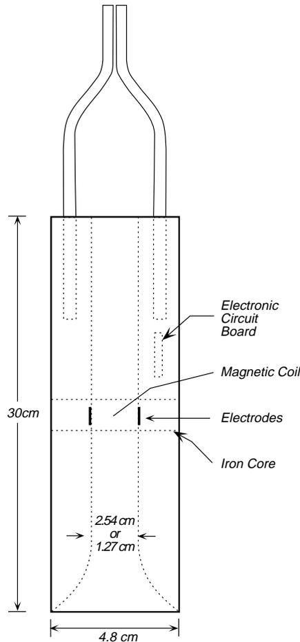
Figure 1. Schematic diagram of the Tennessee Valley Authority electromagnetic borehole flowmeter.
