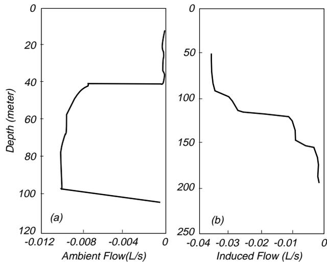
**Figure 3.** Diagrams illustrating the ambient flow distribution in a well and the flow distribution induced by pumping.
