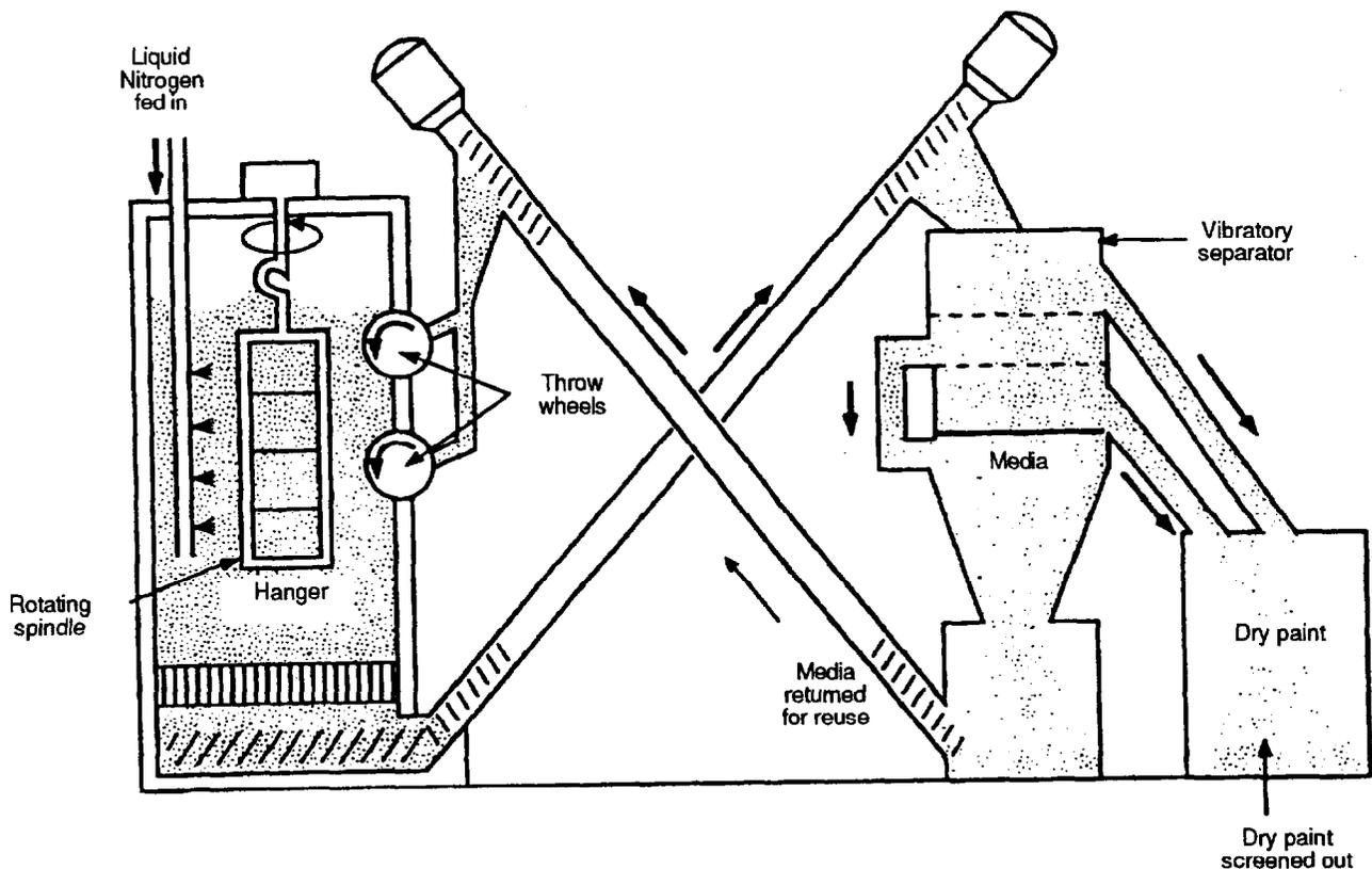
Figure 4. Operation of cryogenic coating removal process equipment.
