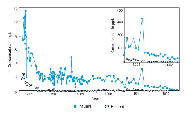
Figure 30. Influent and effluent VOC concentrations (mg/L) at the Chem-Dyne treatment plant from 1987 to 1992 (Cohen et al., 1994, after Papadopulos & Associates, 1993).
