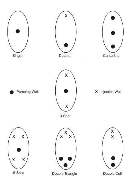
**Figure 23.** Major types of pumping/injection well patterns (Satkin and Dedicate 4000) Bedient, 1988).
