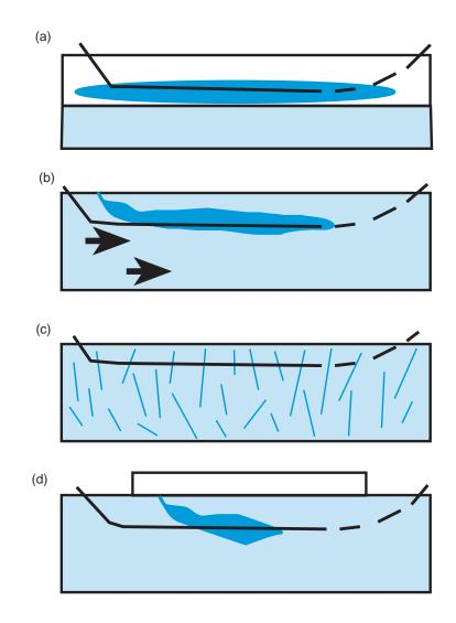
Figure 34. Some applications of horizontal wells: (a) intersecting flat-lying layers, (b) intercepting plume elongated by regional gradient, (c) intersecting vertical fractures, and (d) access beneath structures (U.S. EPA, 1994).
