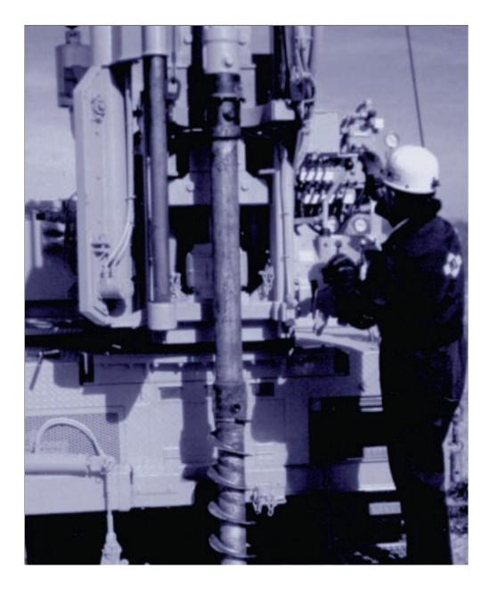
Figure 3. This hollow-stem auger is fitted with a 5-foot sampling tube that collects a advances, allowing detailed and accurate observation of bubble validh of subsurface lithology. When drilling is completed, a monitoring well also can be installed.
