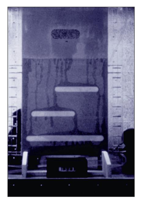
**Figure 12.** Laboratory model of the transport of DNAPL contaminant through an aquifer with varying permeability; note the concentration of downward movement in fingers and the DNAPL pools above the low-permeability zones (the horizontal discs). (Source: U.S. EPA National Risk Management Research Laboratory.)
