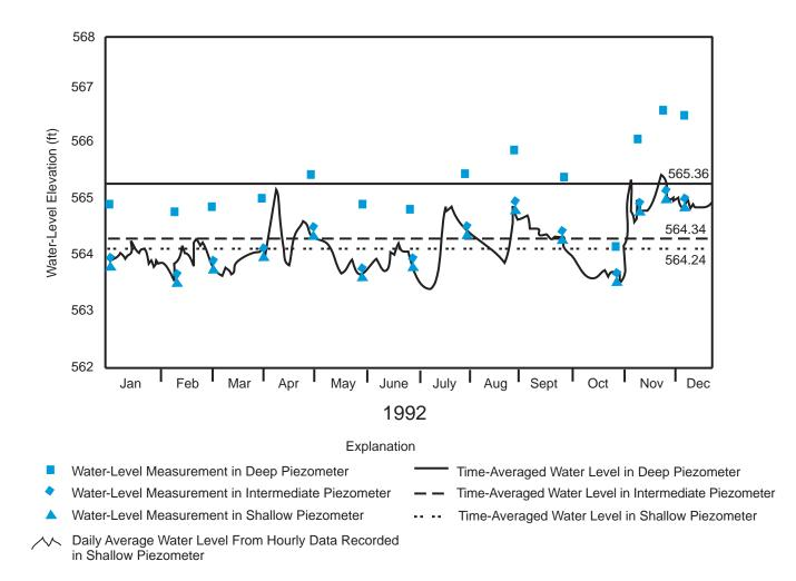
Figure 27. Nested piezometer hydrograph for 1992 at the Chem-Dyne Superfund site (Cohen et al., 1994, after Papadopulos & Associates, 1993).
