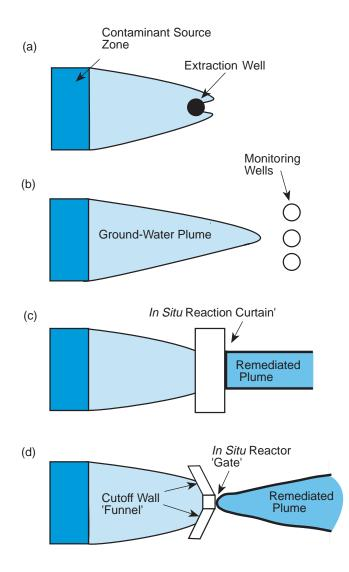
Figure 39. Alternative ground-water plume management options: (a) pump-and-treat system, (b) intrinsic bioremediation, (c) *in situ* reaction curtain, (d) funnel-and-gate system (adapted from Starr and Cherry, 1994).
