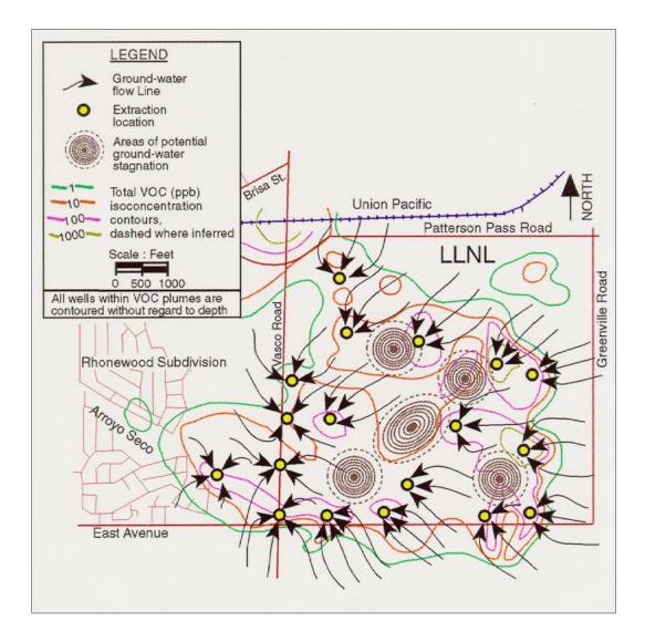
**Figure 24.** Ground-water flow line in the vicinity of conceptual pumping centers at Lawrence Livermore National Laboratory superimposed on an isoconcentration contour map and showing areas of potential stagnation (Cohen et al., 1994, after Hoffman, 1993).
