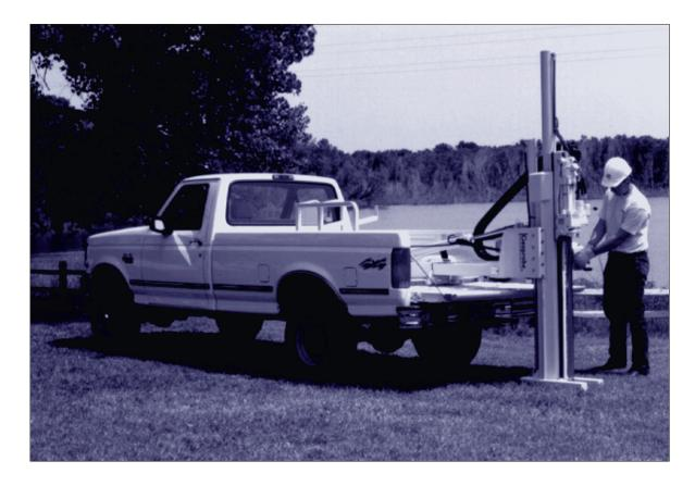
**Figure 4.** Hydraulic or vibratory direct-push rigs can be installed on vans, small trucks, all-terrain vehicles, or trailers and allow collection of continuous soil cores and depth-specific ground-water samples for detailed subsurface mapping if contaminants are generally confined to depths of less than 15 meters. (Photo courtesy of Geoprobe Systems.)
