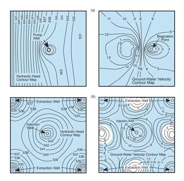
Figure 22. Examples of stagnation zones (shaded where ground-water velocity is less than 4 L/T): (a) single pumping well and (b) four extraction wells with an injection well in the center (Cohen et al., 1994).
