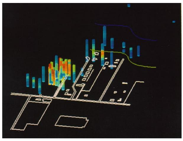
Figure 7. EPA's SITE3D software, under development at the Ada, Oklahoma, laboratory, helps visualize in threedimensions a TCE contaminant plume at a Superfund Site. Yellows and reds indicate zone with highest concentrations of TCE in ground water.
