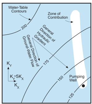
Figure 20. Effect of fracture anisotropy on the orientation of the zone of contribution (capture zone) to a pumping well (Bradbury et al., 1991).
