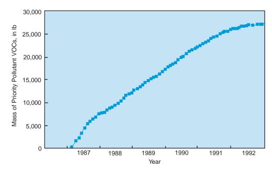
Figure 31. Cumulative mass of VOCs removed from the aquifer at the Chem-Dyne site from 1987 to 1992 (Cohen et al., 1994, after Papadopulos & Associates, 1993).
