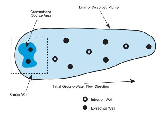
**Figure 17.** Plan view of a mixed containment-restoration strategy. A pump-and-treat system is used with barrier walls to contain the ground-water contamination source areas (e.g., where NAPL or waste may be present) and then collect and treat the dissolved contaminant plume (Cohen et al., 1994).
