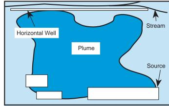
Figure 35. Two approaches using trenches or horizontal wells to intercept contaminant plumes (U.S. EPA, 1994).
