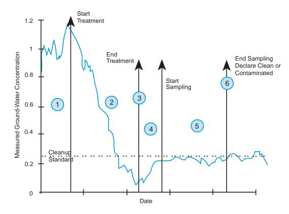
Figure 33. Stages of remediation in relation to example contaminant concentrations in a well at a pump-and-treat site (U.S. EPA, 1992).
