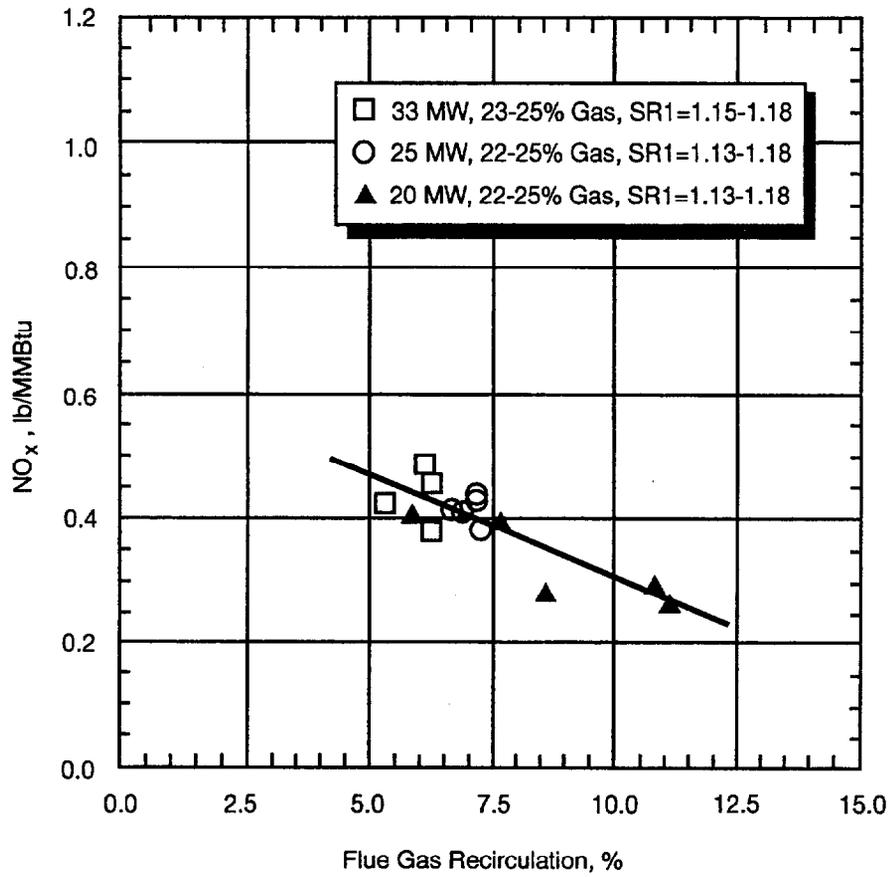
Figure 3-14. Lakeside Unit 7—Effect of Flue Gas Recirculation on NO<sub>x</sub> Emissions (Folsom et al., 1994).
