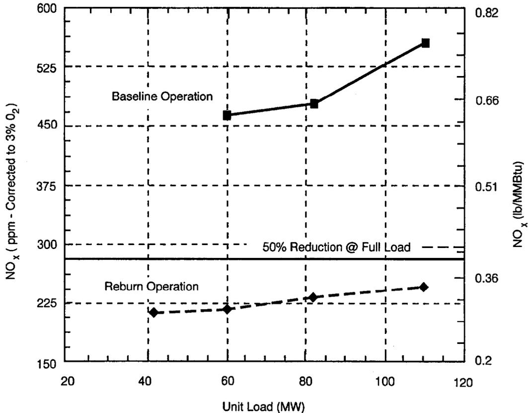
Figure 3-18. Nelson Dewey Unit 2-NO<sub>x</sub> Emissions vs. Unit Load - Powder River Basin Coal (Newell et al., 1993).
