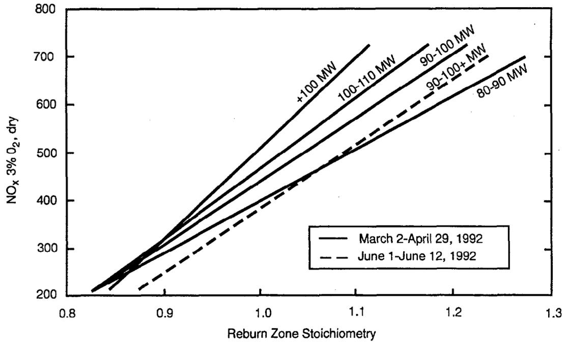
Figure 3-20. Niles Unit 1-Variation of NO<sub>x</sub> with Reburn Stoichiometry (Borio et al., 1993).
