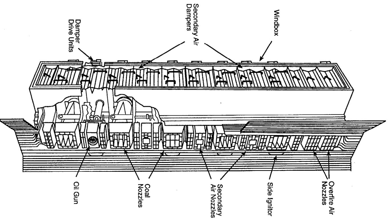
Figure 2-7. Burner Assembly of a Tangentially-Fired Boiler (Singer, 1991).
