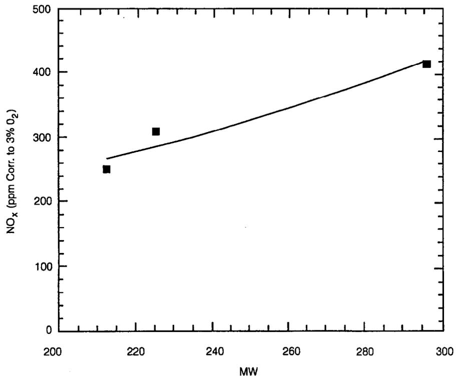
Figure 3-25. Ladyzhin Unit 4-NO<sub>x</sub> Emissions vs. Boiler Load.
