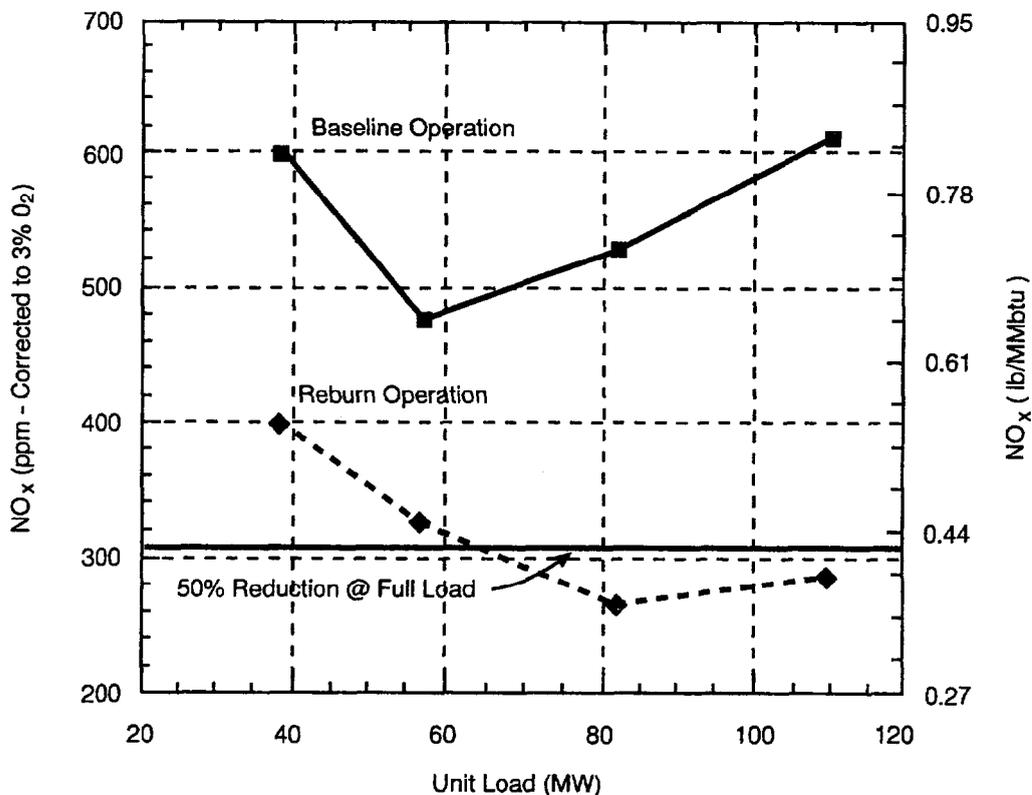
Figure 3-17. Nelson Dewey Unit 2-NO<sub>x</sub> Emissions vs. Unit Load - Illinois Basin Coal (Newell et al., 1993).
