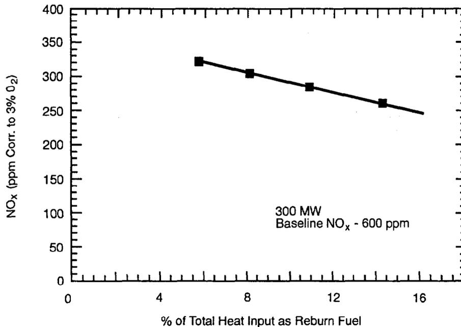
Figure 3-23. Ladyzhin Unit 4-NO<sub>x</sub> Emissions vs. Reburn Fuel Percentage (LaFlesh et al., 1993).
