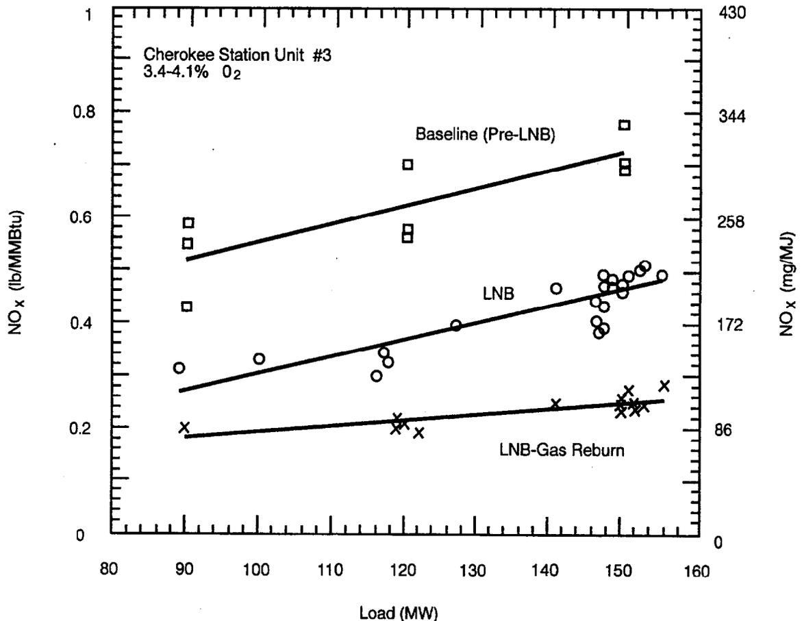
Figure 3-6. Cherokee Unit 3—Effect of Unit Load on NO<sub>x</sub> Emissions (Sanyal et al., 1993).
