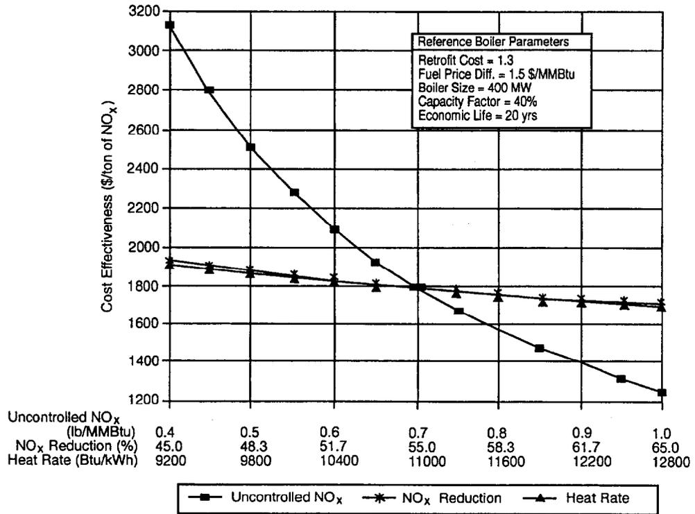
Figure 4-4. Impact of NO<sub>x</sub> Emission Characteristics and Heat Rate on Return Cost Effectiveness for Tangentially-Fired Boilers (U.S. EPA, 1994).
