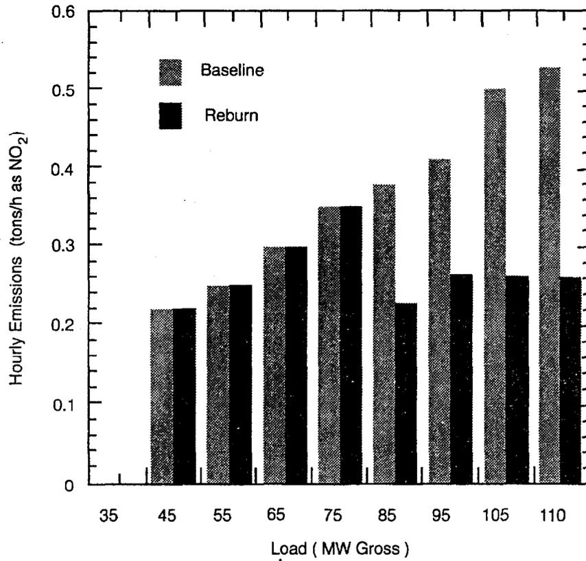
Figure 3-21. Niles Unit 1-NO<sub>x</sub> Emissions as a Function of Boiler Load (Borio et al., 1993).
