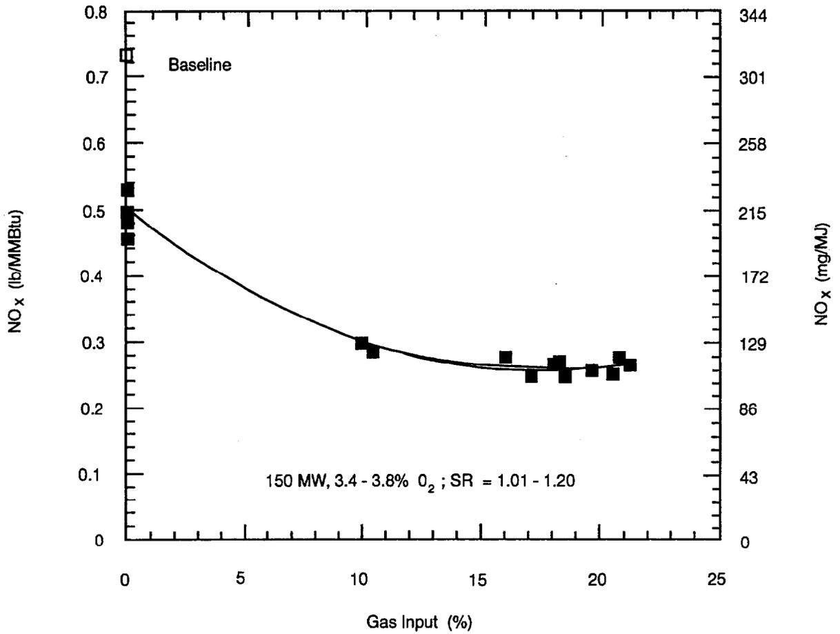
Figure 3-5. Cherokee Unit 3—Effect of Gas Input on NO<sub>x</sub> Emissions (Sanyal et al., 1993).
