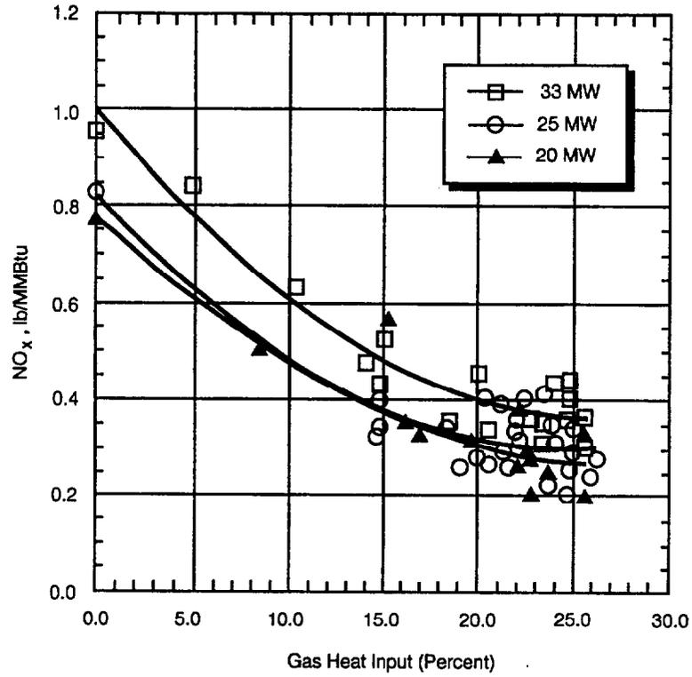
Figure 3-12. Lakeside Unit 7—Effect of Gas Heat Input on NO<sub>x</sub> Emissions (Folsom et al., 1994).
