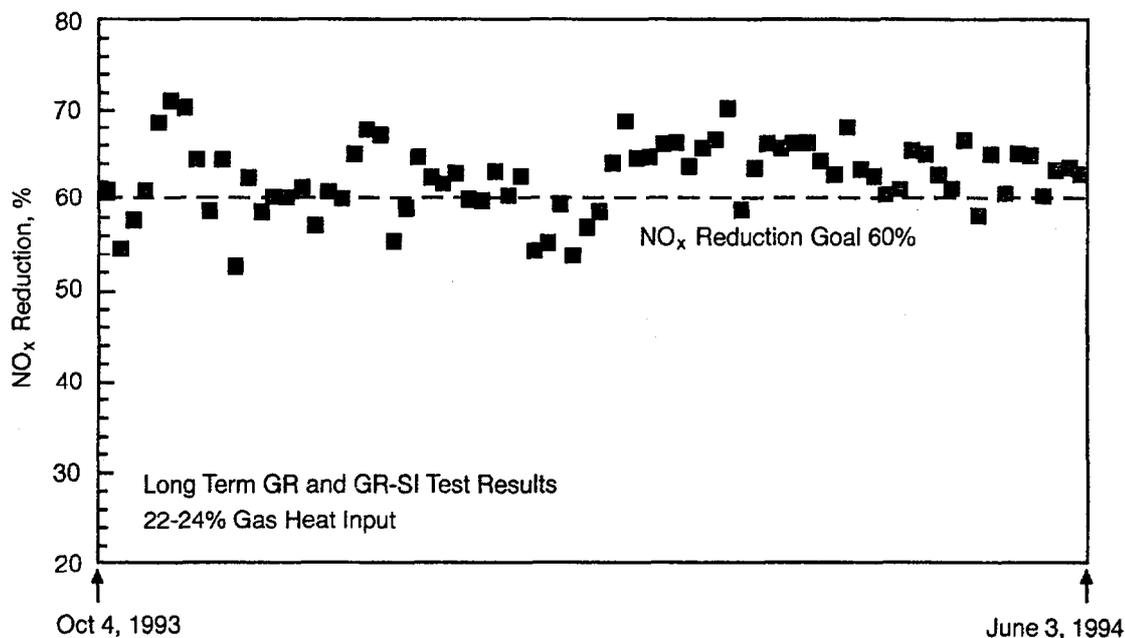
Figure 3-15. Lakeside Unit 7-Long-Term Operation Results for  $\text{NO}_x$  Reductions (Folsom et al., 1994).
