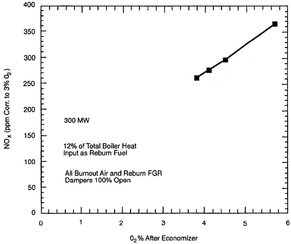
Figure 3-24. Ladyzhin Unit 4-NO<sub>x</sub> Emissions vs. Flue Gas Oxygen Content.
