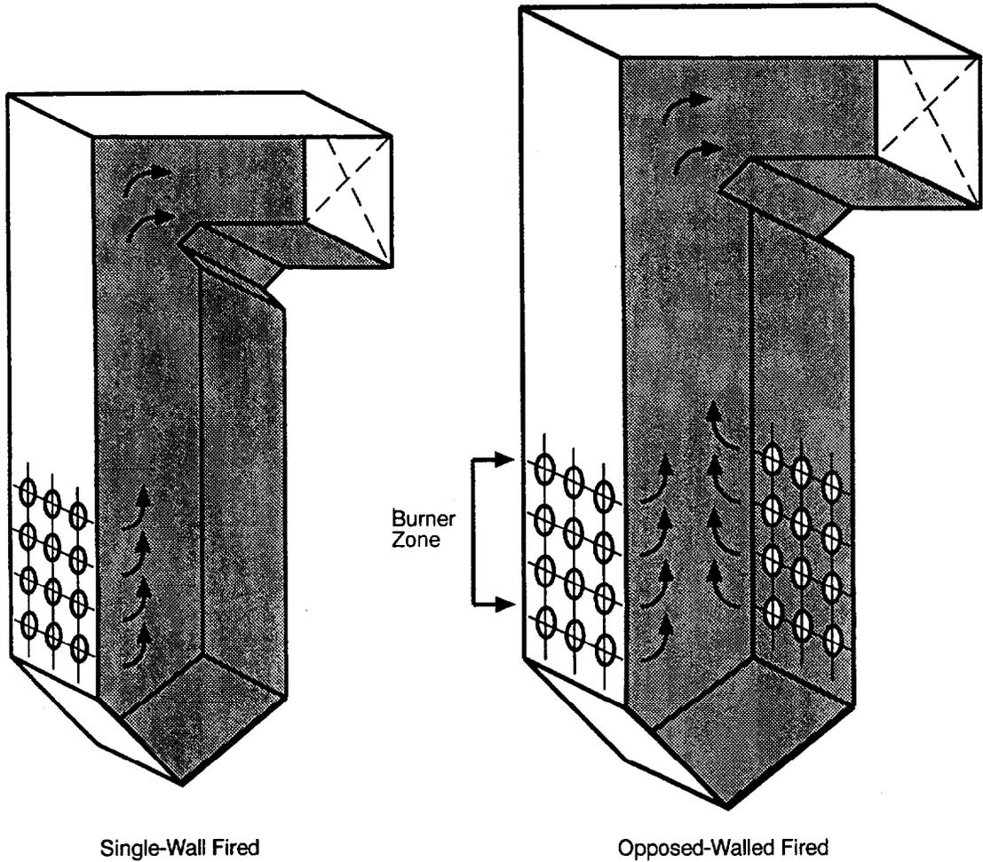
Figure 2-8. Single-Wall and Opposed-Wall Type Wall-Fired Boilers.
