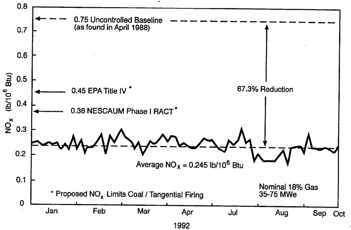
Figure 3-10. Hennepin Unit 1—Long-Term Gas Reburning Data (Folsom et al., 1993).
