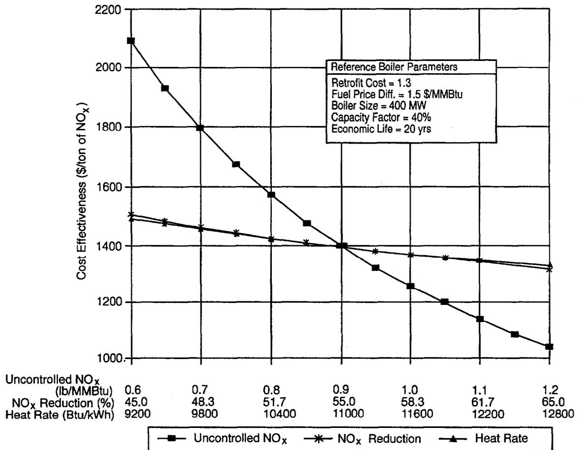
Figure 4-2. Impact of NO<sub>x</sub> Emission Characteristics and Heat Rate on Reburn Cost Effectiveness for Wall-Fired Boilers (U.S. EPA, 1994).
