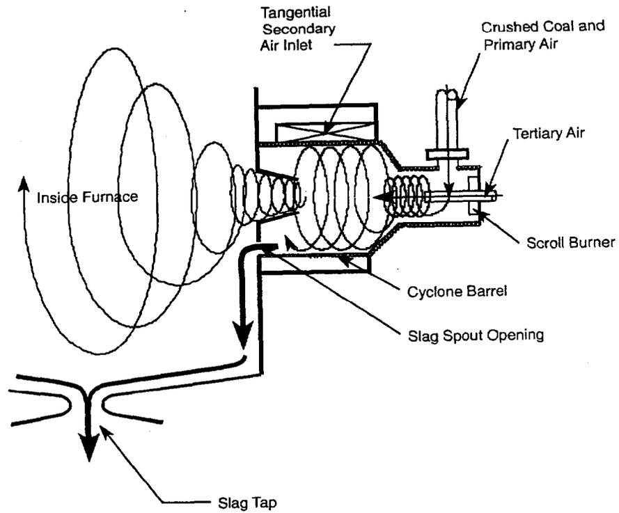
Figure 2-12. Cyclone Burner (Farzan, et al., 1991).
