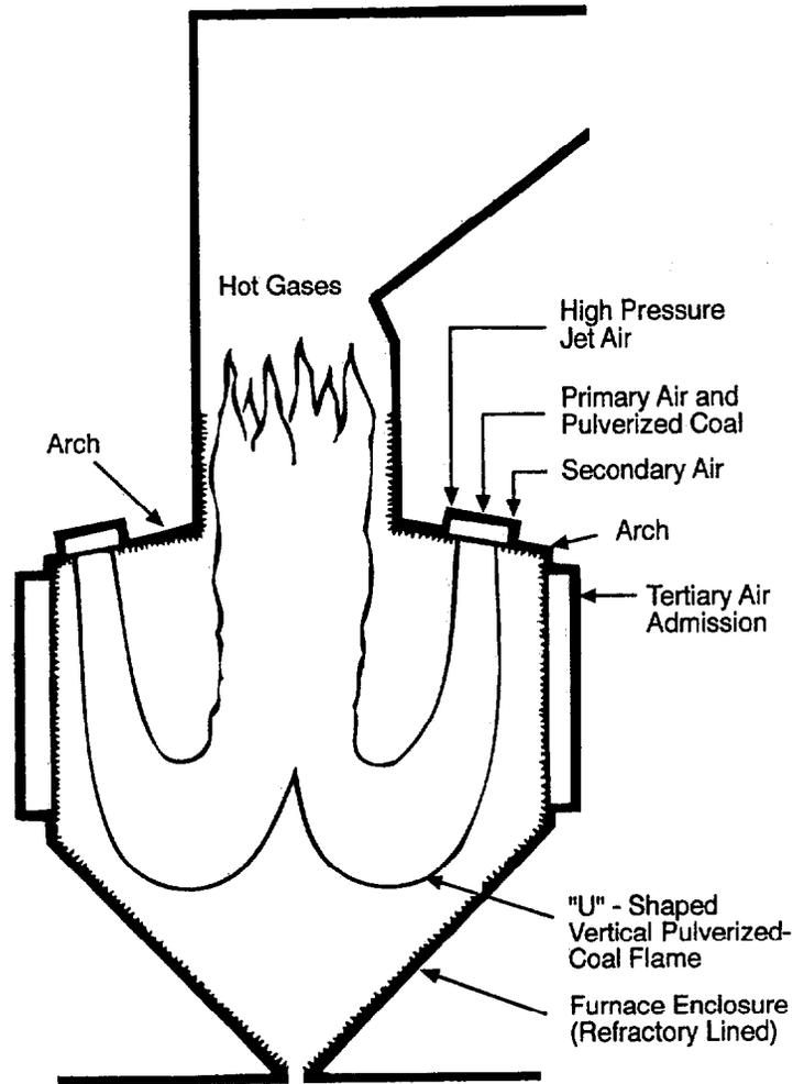
Figure 2-11. Flow Pattern in an Arch-Fired Boiler (Singer, 1991).
