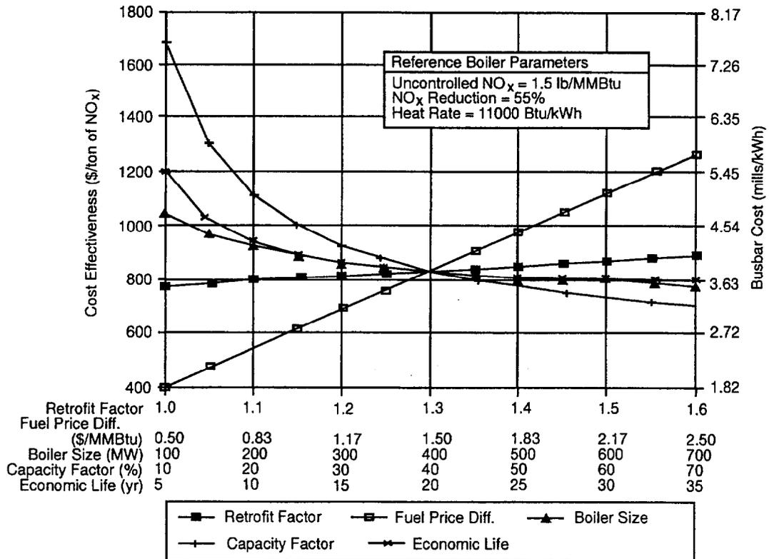
Figure 4-5. Impact of Plant Characteristics on Return Cost Effectiveness and Busbar Cost for Cyclone-Fired Boilers (U.S. EPA, 1994).
