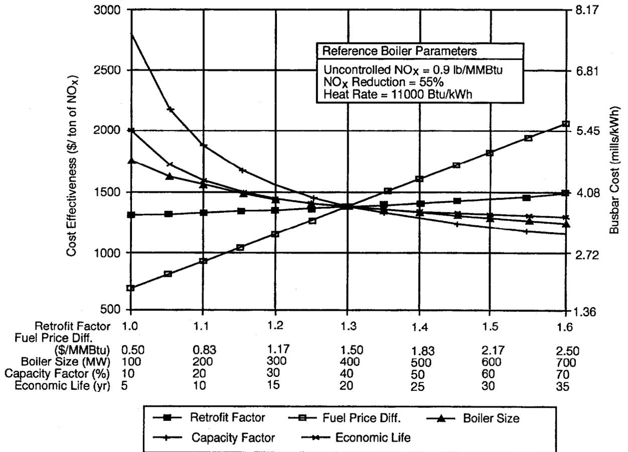
Figure 4-1. Impact of Plant Characteristics on Return Cost Effectiveness and Busbar Costs for Wall-Fired Boilers (U.S. EPA, 1994).
