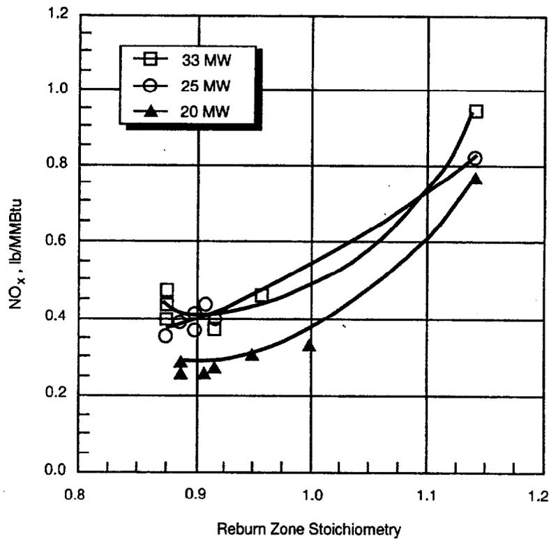
Figure 3-13. Lakeside Unit 7—Effect of Reburn Zone Stoichiometry on NO<sub>x</sub> Emissions (Folsom et al., 1994).
