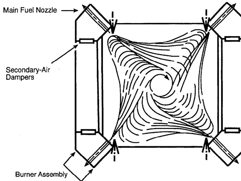
Figure 2-6. Firing Pattern in a Tangentially-Fired Boiler (Singer, 1991).
