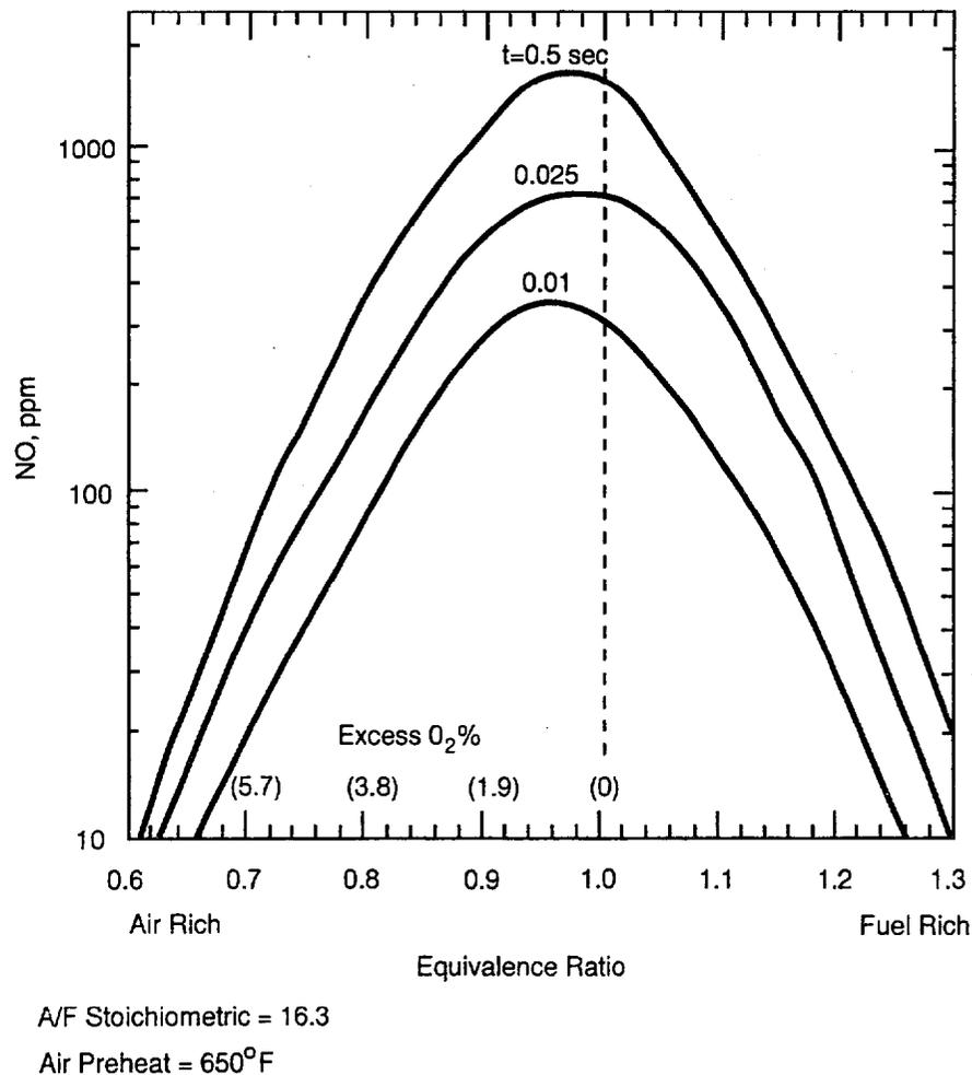
Figure 2-1. Effect of Equivalence Ratio on NO<sub>x</sub> Formation (Bagwell, et al. 1971).
