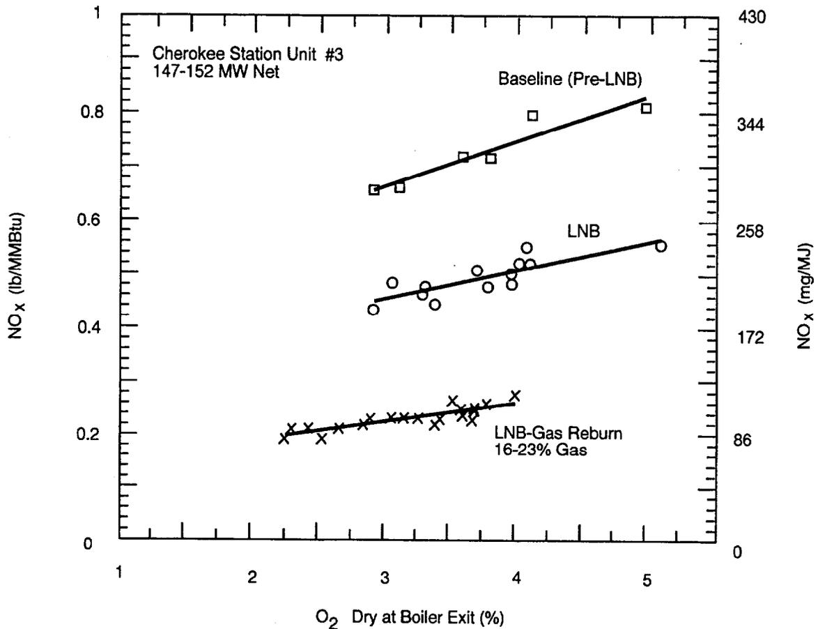
Figure 3-4. Cherokee Unit 3—Effect of Excess Air on NO<sub>x</sub> Emissions (Sanyal et al., 1993).
