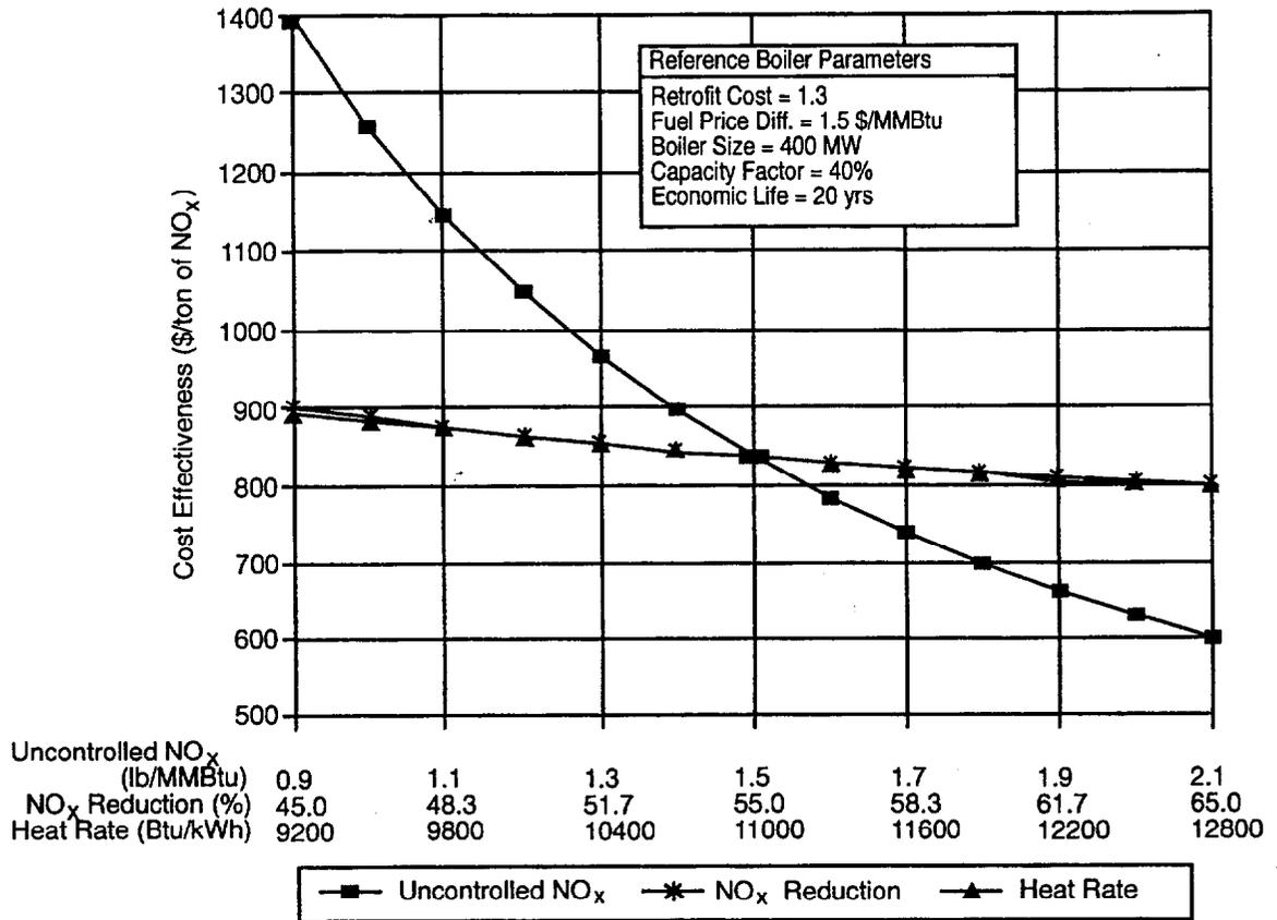
Figure 4-6. Impact of NO<sub>x</sub> Emission Characteristics and Heat Rate on Return Cost Effectiveness for Cyclone-Fired Boilers (U.S. EPA, 1994).
