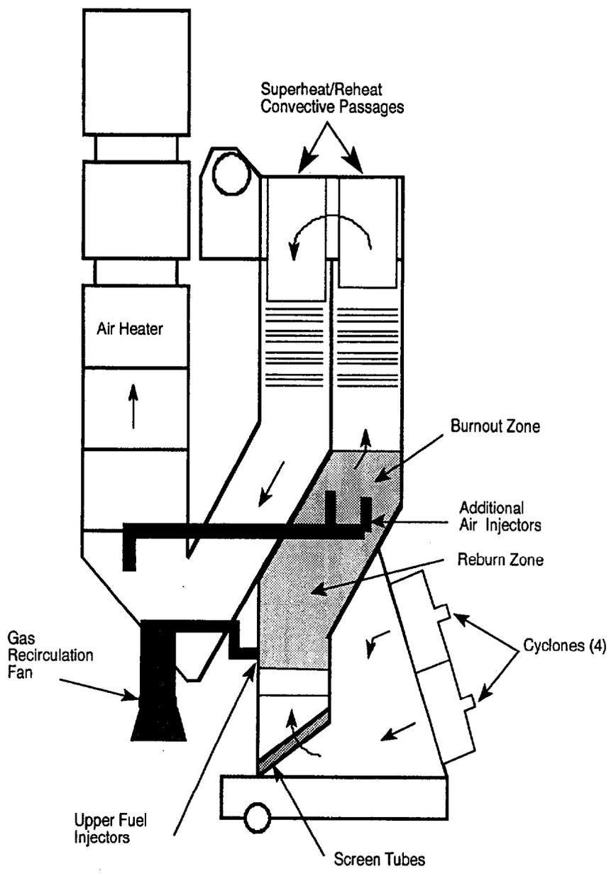
Figure 3-19. Niles Unit 1—Schematic of Reburn Process (Borio et al., 1993).
