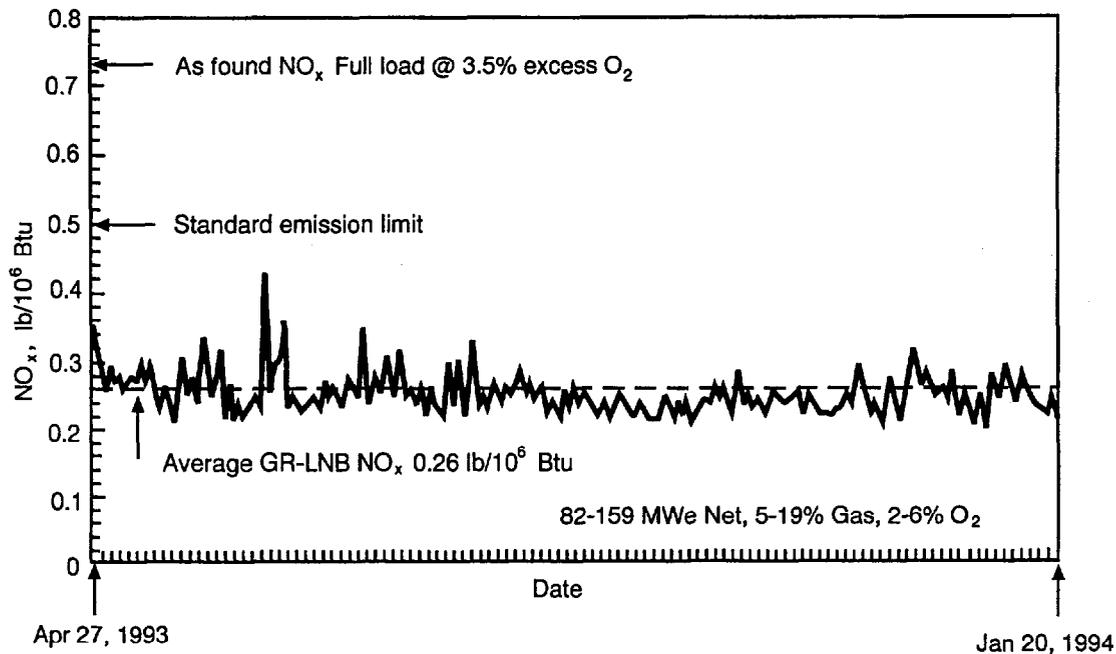
Figure 3-7. Cherokee Unit 3—Long-Term NO<sub>x</sub> Emission Data (Sanyal et al., 1993).
