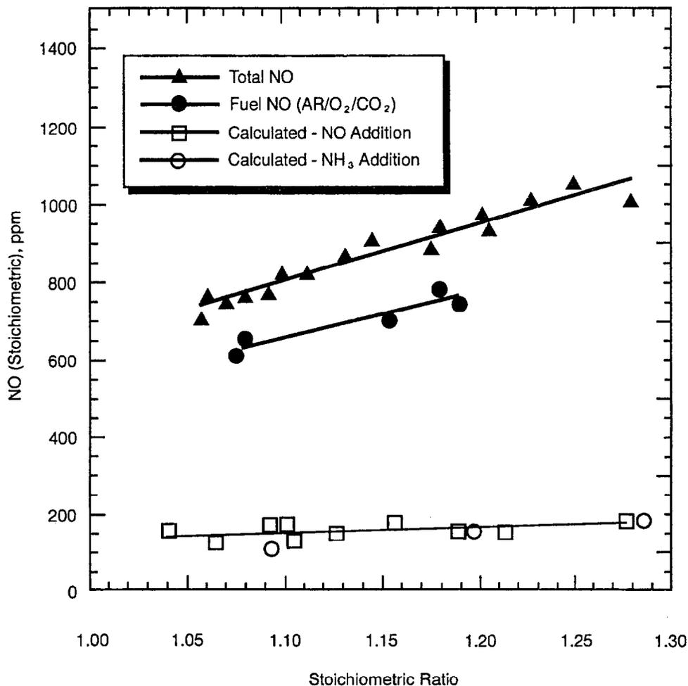
Figure 2-4. Sources of NO<sub>x</sub> Emissions from Coal (Pershing and Wendt, 1976).
