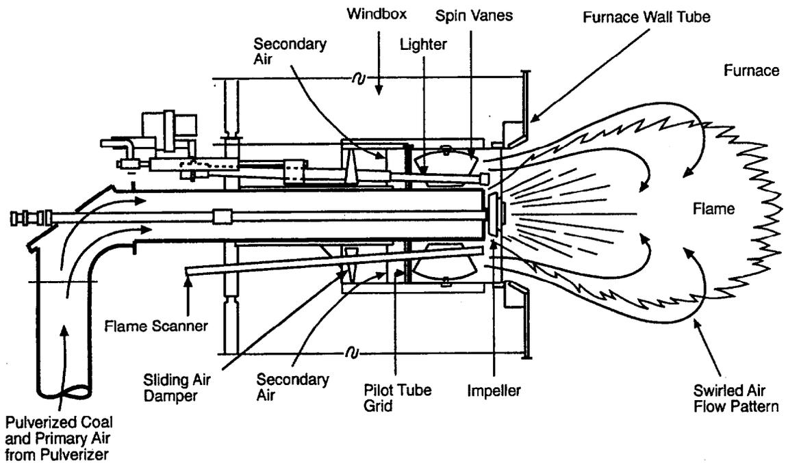
Figure 2-9. Typical Circular Burner (Stultz and Kitto, 1992).
