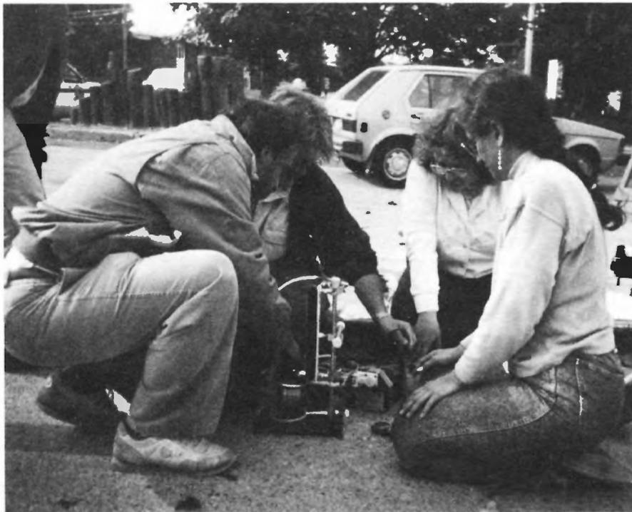
Students at EPA's "Soil Vapor Boot Camp" sample and analyze gasoline tank leaks. The service station they are testing, on the University of Connecticut-Storrs campus, was the scene of an actual leak.
