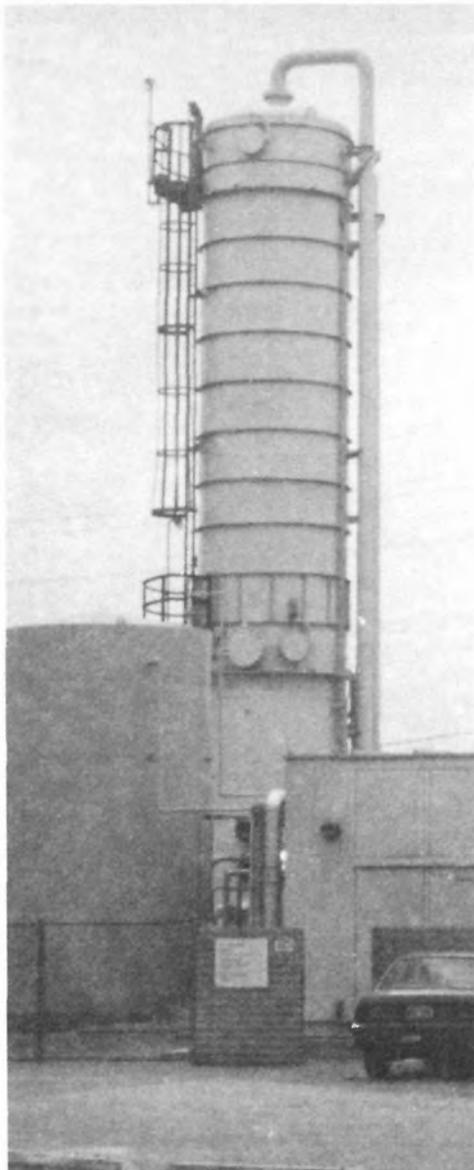
*AWD AquaDetox/SVE System: Simultaneously treats ground water and soil gas in closed loop system that eliminates air emissions. Proprietary moderate-vacuum steam stripping tower removes organics from ground water; soil vapor extraction (SVE) system removes soil gas for subsequent treatment with granular activated carbon beds.*
