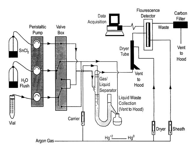
Figure 1: Automated Mercury Fluorescence System
