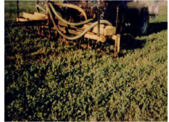
Even liquid manure application by drag line incorporation.
