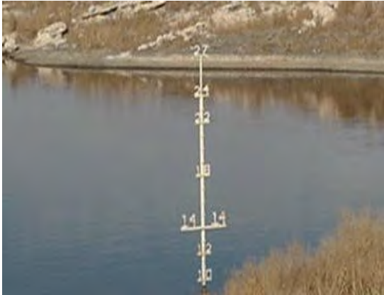
Depth markers gauge runoff holding pond levels and help avoid capacity issues.
