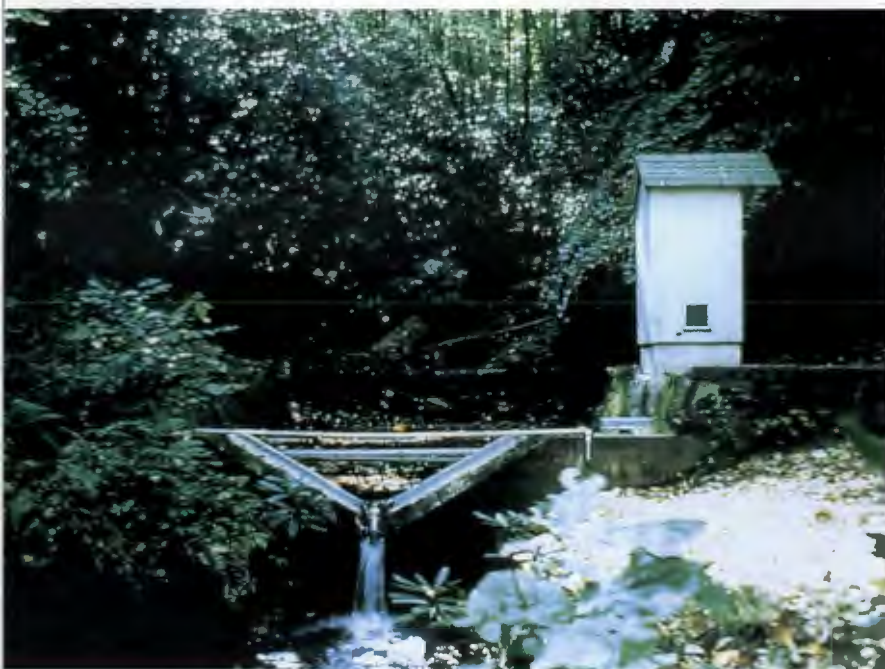
Figure 7.9: Station measuring discharge. Permanent stations provide measurements for a wide range of flow, but the necessary measurements can be made in other ways. Source: C. Zabawa.
