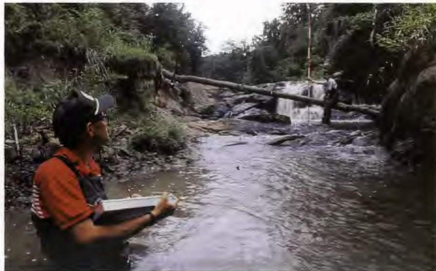
Figure 8.49: Surveying a stream. Channel surveys establish baseline information needed for restoration design.
