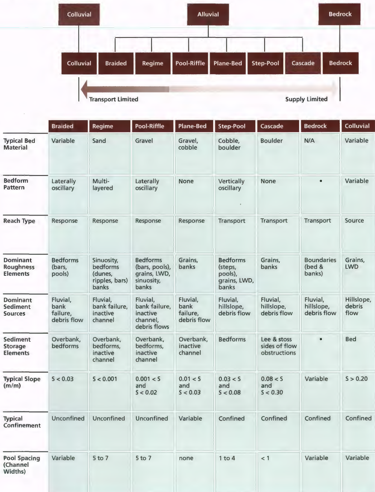
Figure 7.11: Suggested stream classification system for Pacific Northwest. Included are classifications for nonalluvial streams. Source: Montgomery and Buffington 1993.
