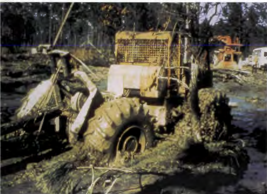
Figure 9.9: Lessons to be learned. Heavy equipment can quickly reduce a vegetated area to churned earth.
