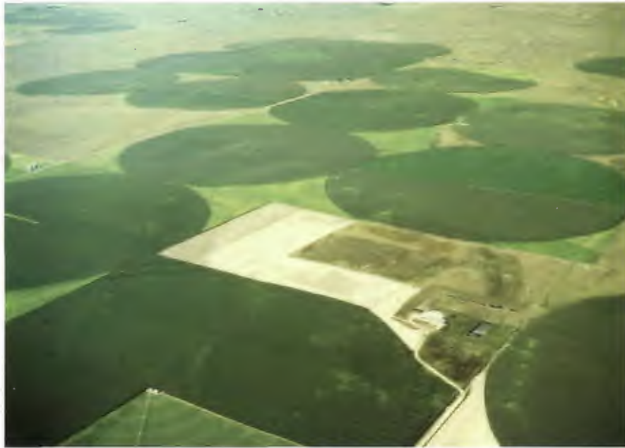
Figure 3.15: Central pivot irrigation systems use ground water sources. Reliance on aquifers for irrigation has brought about major changes in ground water supply, as well as the landscape.
