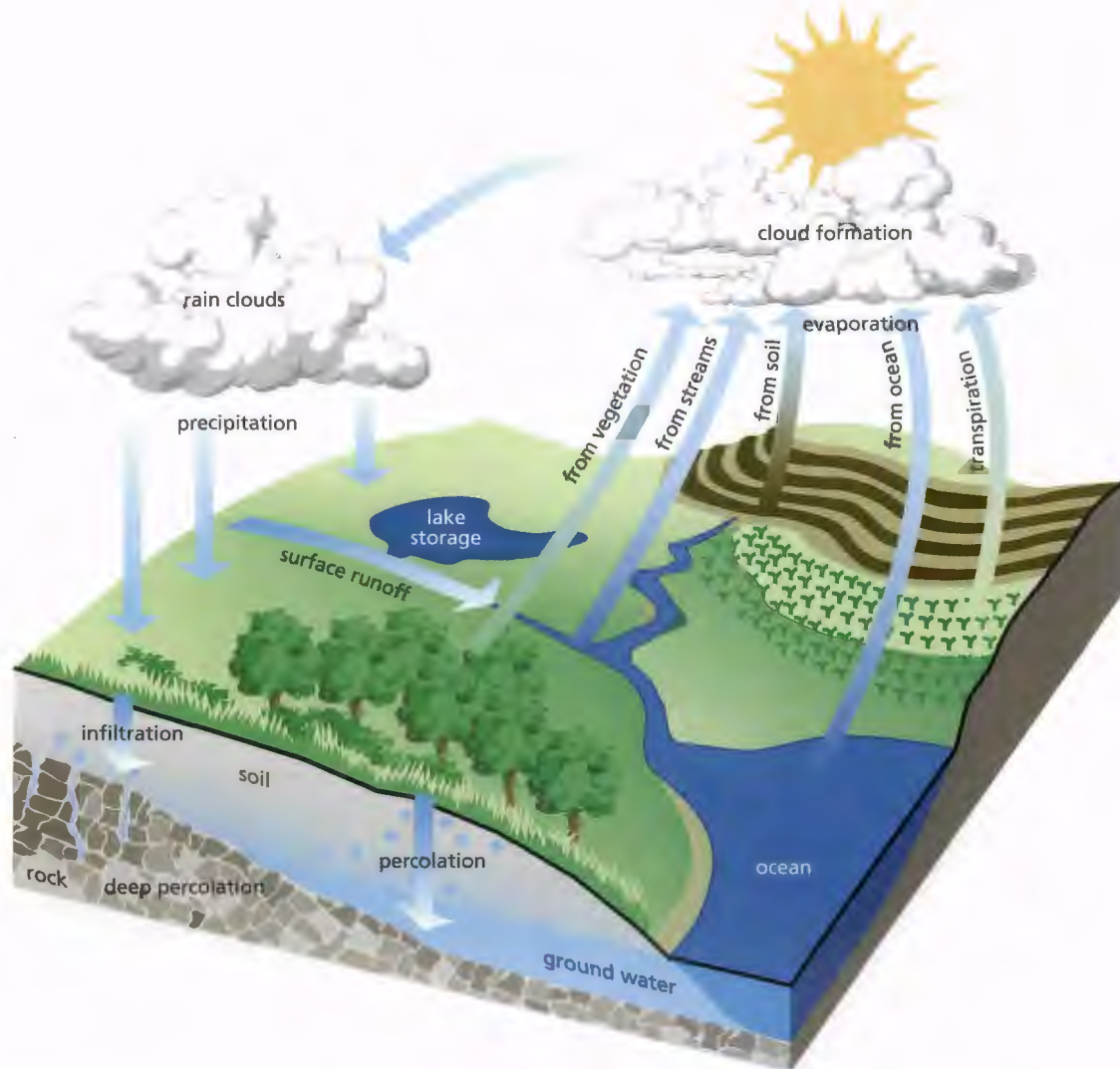
Figure 2.2: The hydrologic cycle. The transfer of water from precipitation to surface water and ground water, to storage and runoff, and eventually back to the atmosphere is an ongoing cycle.
