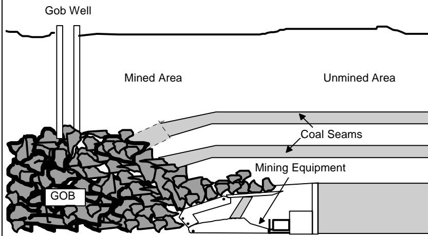
is pulled on the well in most cases to prevent methane from entering mine working areas. Exhibit 4-3 presents a schematic of a gob well.
