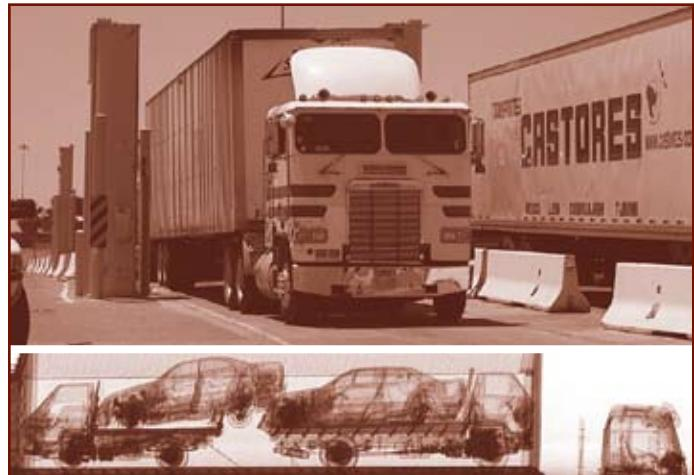
*Increasing sophisticated technology is being applied to scan incoming cargo for unauthorized contents. Shown are: (1) a truck passing through a gamma ray scanner at Otay Mesa port of entry in San Diego (Source: Paul Ganster, San Diego State University); and (2) a radiographic image showing stolen vehicles that has been installed in a port of entry office (Source: SAIC).*
