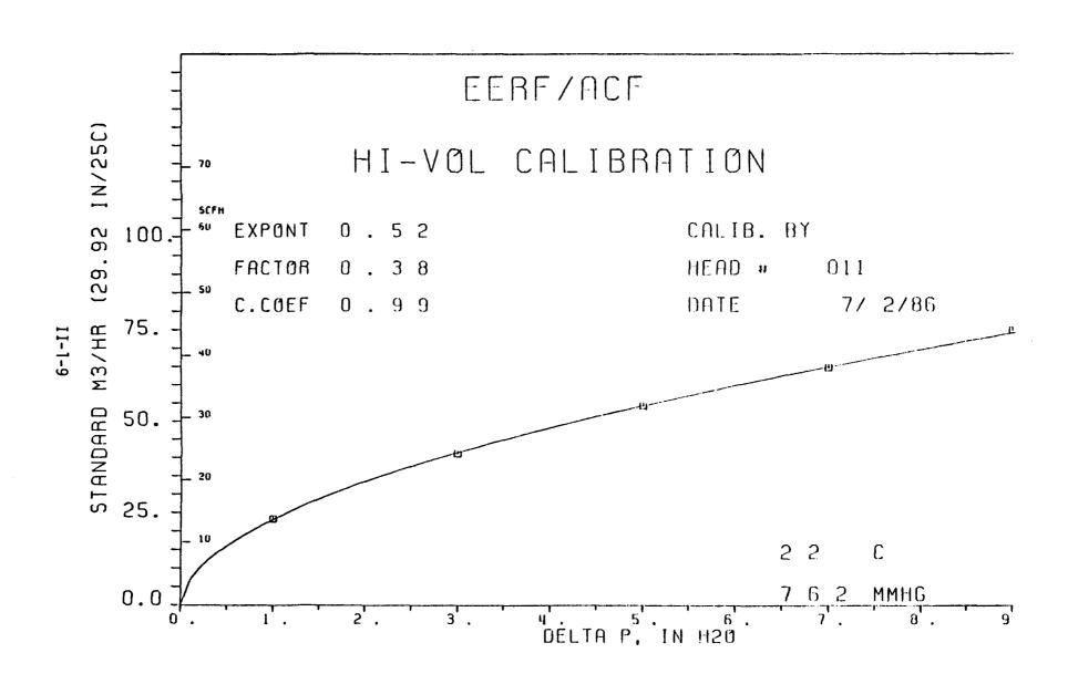
To determine the total air volume moved through the filter, the average flow rate is multiplied by the sampling time in hours.
