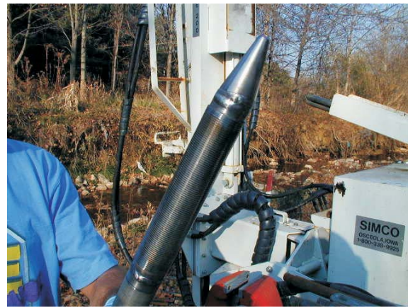
Figure 8. Stainless steel piezometer used in piezometer nests.
