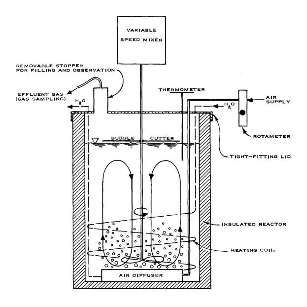
Figure 2. Schematic diagram of batch reactor
