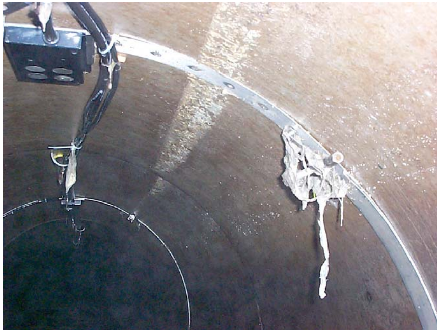
Figure 4-26. Debris accumulation on ADS 4000's bender.
