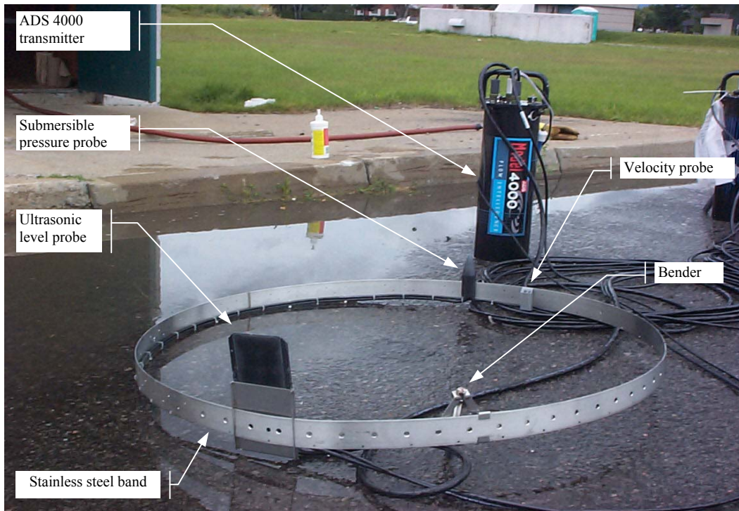
Figure 4-10. ADS 4000 flow meter components.
