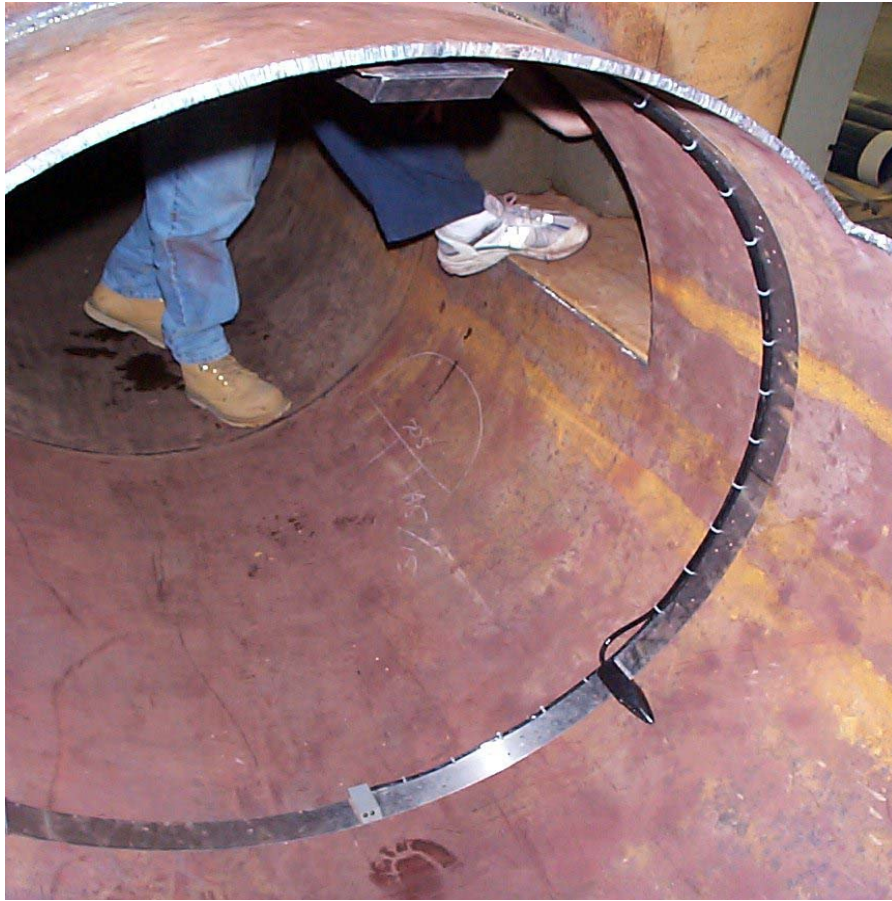
Figure 3-9. ADS flow monitoring sensors (laboratory 42-inch pipe installation).
