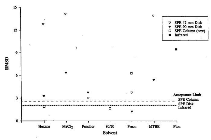
NOTE: Points below the respective Acceptance Limit'are not significantly different from separatory funnel extraction with Freon
