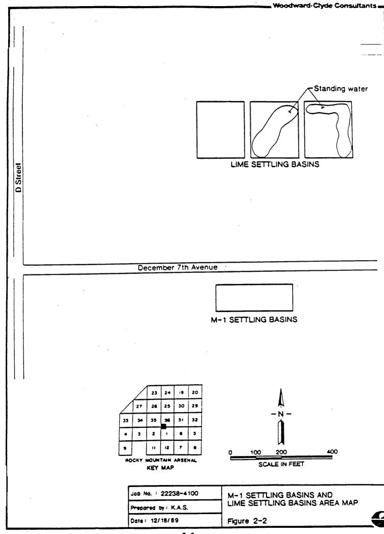
The M-1 Settling Basins were backfilled, probably in 1947, and are now covered with soil. Portions of the basins are covered with structures. These structures will be relocated before implementation of the IRA.
