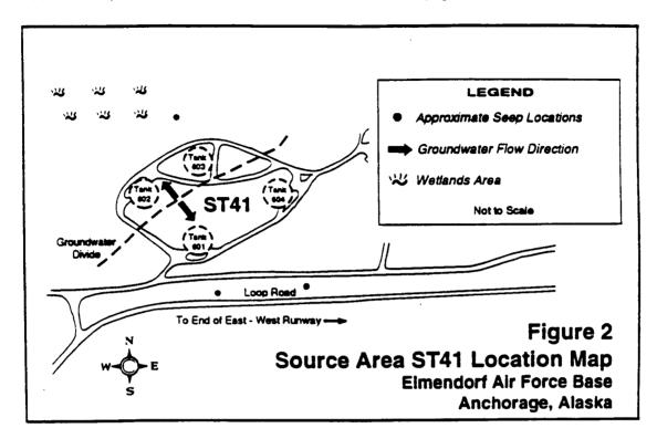
ST41 includes four one-million gallon, underground JP-4 and aviation gasoline storage tanks and ancillary piping constructed in the early 1940s. Reports indicate that the tanks are steel and may have an outer concrete lining. ST41 also includes an area of approximately one acre located west of the tanks which is described as a tank sludge burial area. The sludge burial area will be investigated in the ongoing remedial investigation/feasibility study (RI/FS) for OU2.
