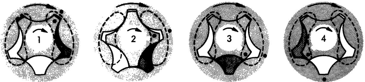
Fig. 5-8 Operating Cycle of Gerotor Pump
