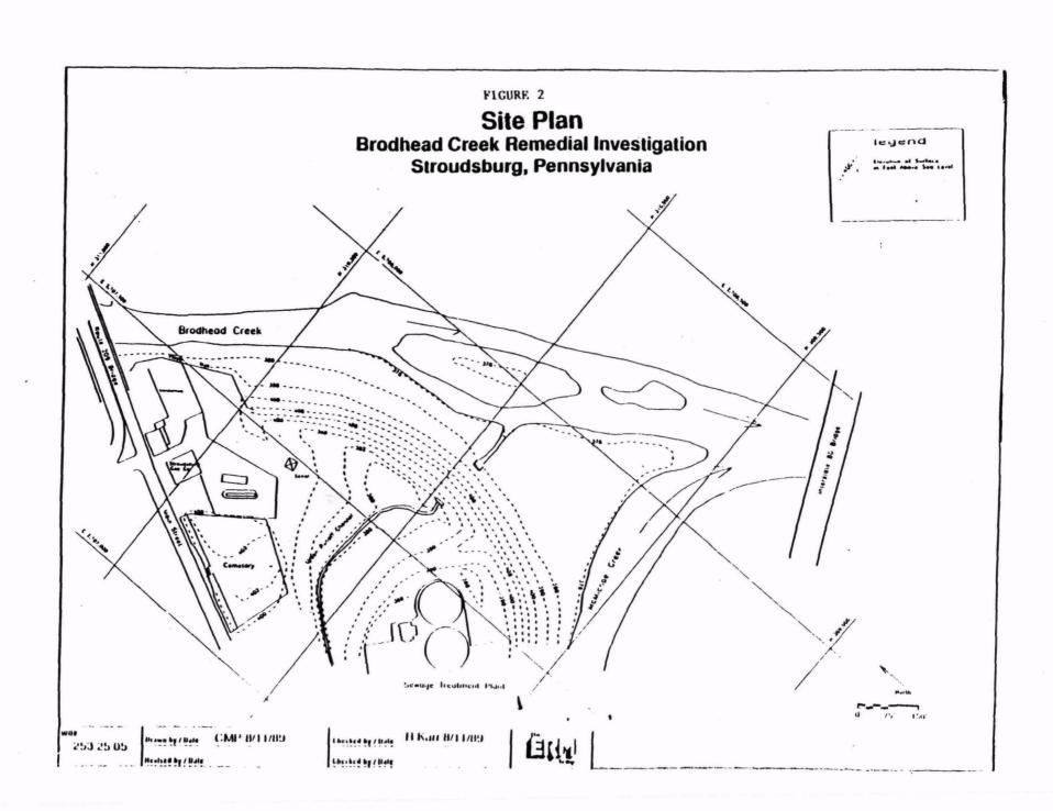
smaller of the two is intermittent in nature, as it carries storm run-off, entering the Site at the northeast corner via a storm sewer outfall. The smaller channel is not considered to be a major Site feature for this reason. The larger channel is perennial in nature and enters the Site from the west-northwest, flowing across the central portion of the Site through a flood gate in the levee to its-outlet on Brodhead Creek. It is referred to herein as the urban run-off channel.
