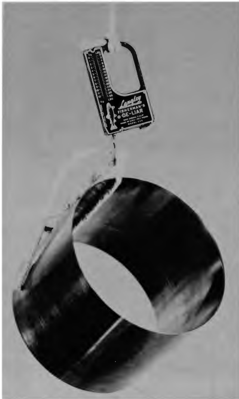
FIGURE 14. Free-Standing Sputtered Copper Cylinder. This deposit, which is over 1/8" thick was removed from its substrate by machining, producing a high-strength cylinder.
