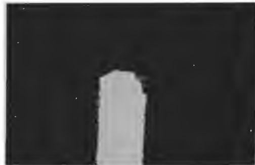
Sputtered 304 stainless steel oxidized in air at 2200°F for 16 hr. Although the composition is the same, the sputter-deposit oxidized much less than the wrought specimen (1.6 mils vs 23 mils). Magnification 30 times.
