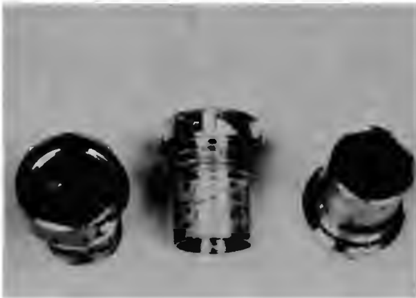
Fig. 18 Electroless plated nickel salt spray test
