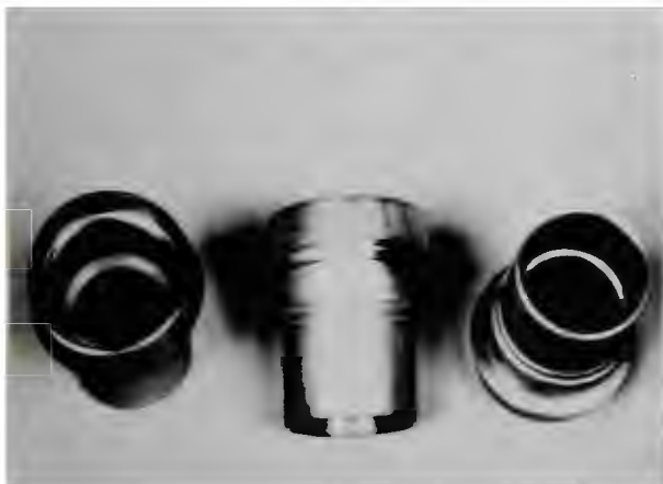
Fig. 16 Electroplated cadmium salt spray test specimens
