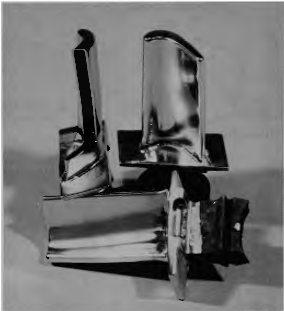
FIGURE 16. Turbine Blades Fabricated by the Soluble Mandrel Method Shown in Figure 15.
