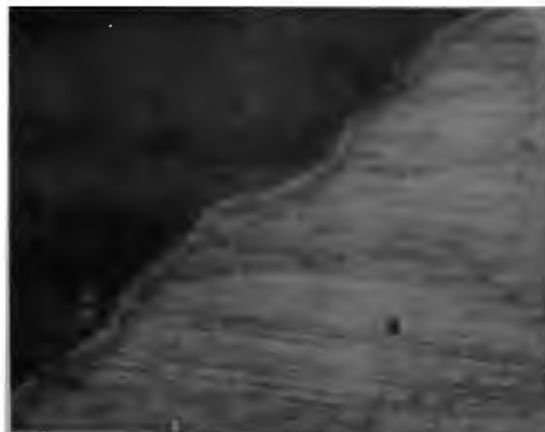
Fig. 5 Section showing IVD Al coating thickness on internal surface 250X
