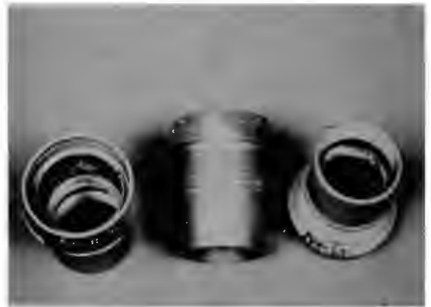
Fig. 19 IVD aluminum coated salt spray test specimens
