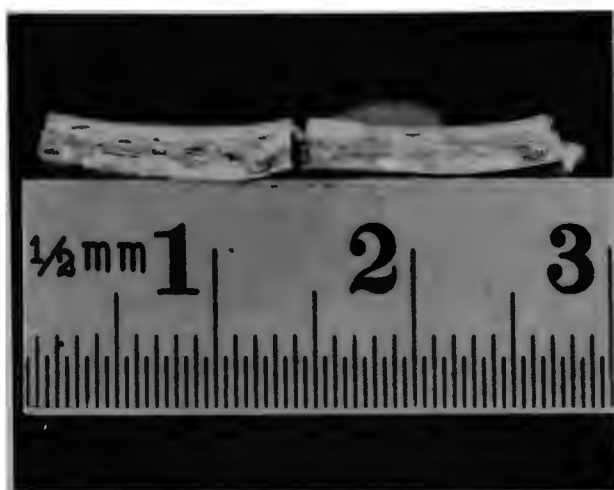
Fig. 10 IVD aluminum coated adhesion test specimens.
