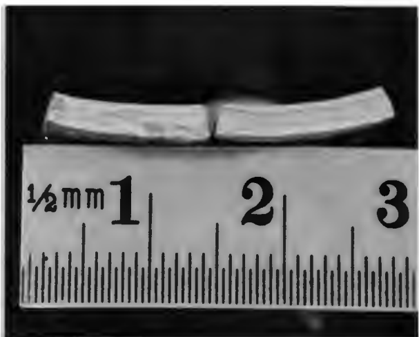
Fig. 9 Zinc flake/chromate mixture coated adhesion test specimens
