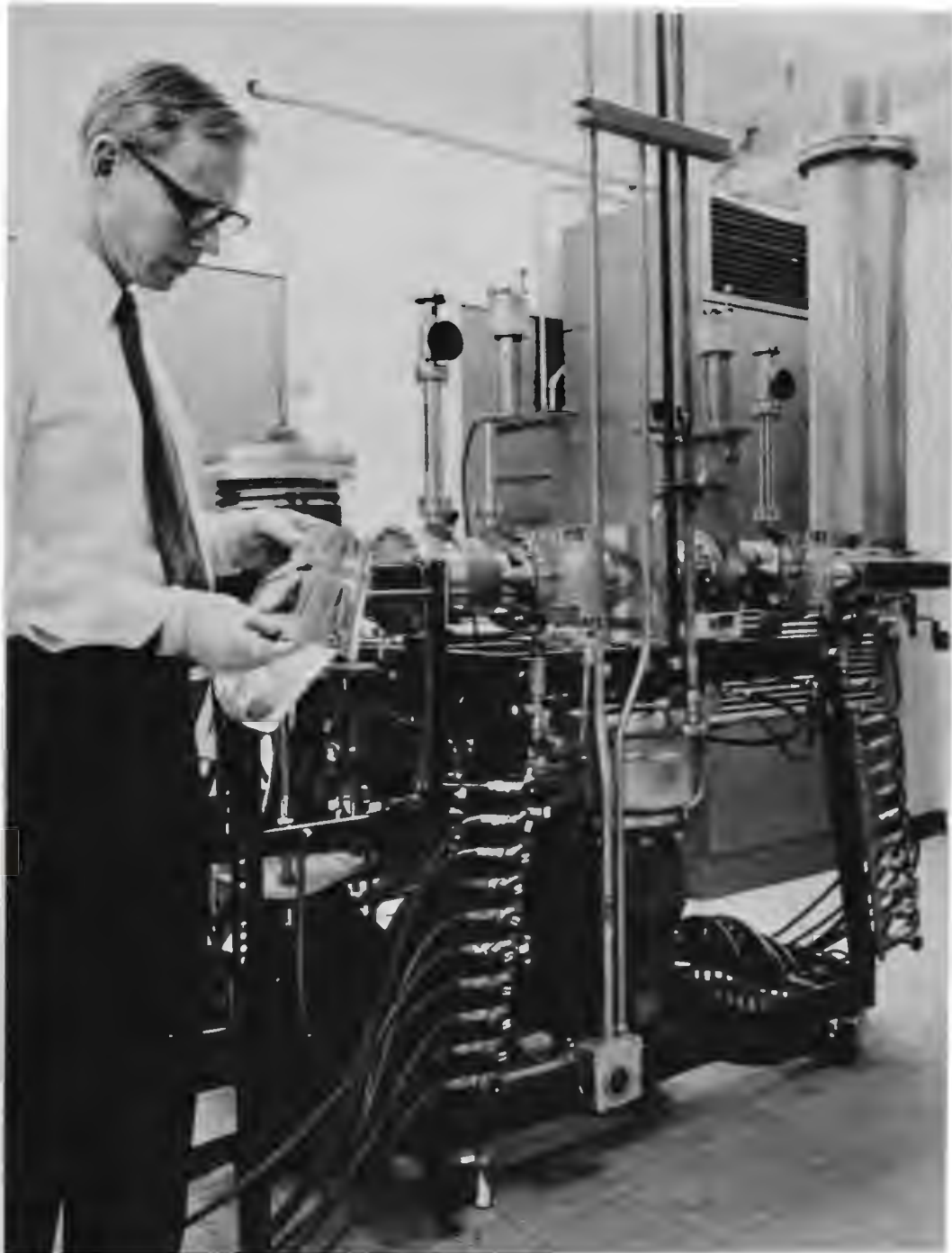
FIGURE 3. BNW Dual-Head Sputtering Apparatus. While a deposition is being performed on one end, the other is being prepared. Note the oil diffusion pump, cold trap, dual gate valves, ports for an RGA and cooling water manifold. The deposit being held is copper foil whose substrate was a pyrex pipe.
