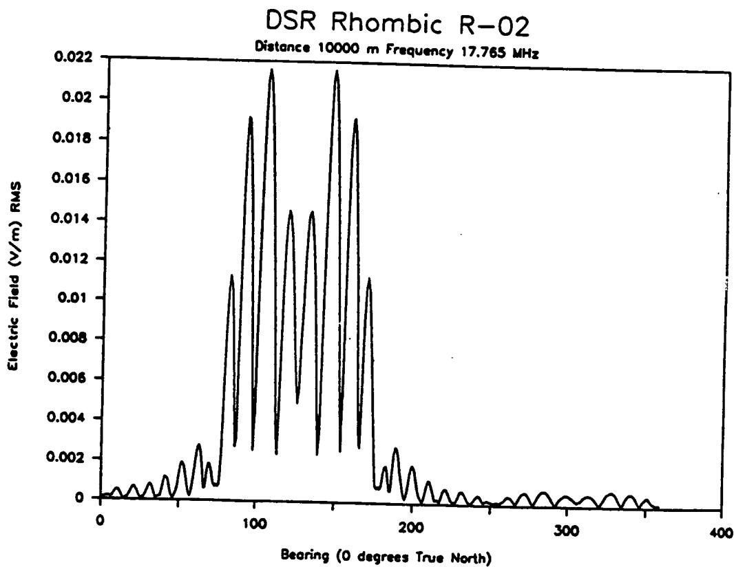
Figure 26. Calculated Electric Field for Rhombic R-02 at 17.765 MHz.
