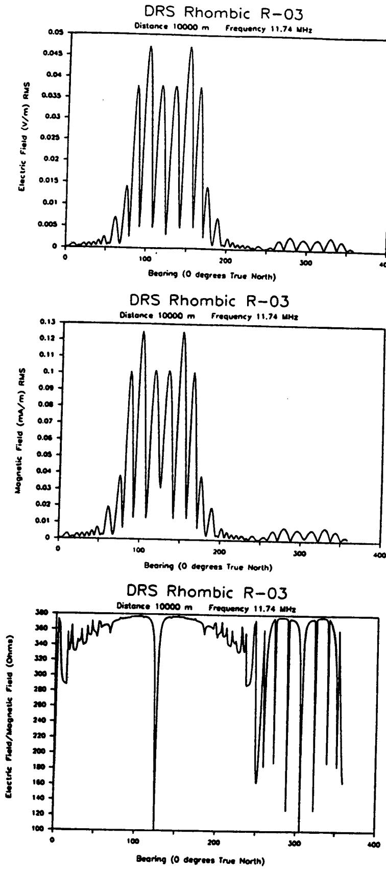
Figure 23. Calculated Fields for Rhombic R-03 at 11.74 MHz.
