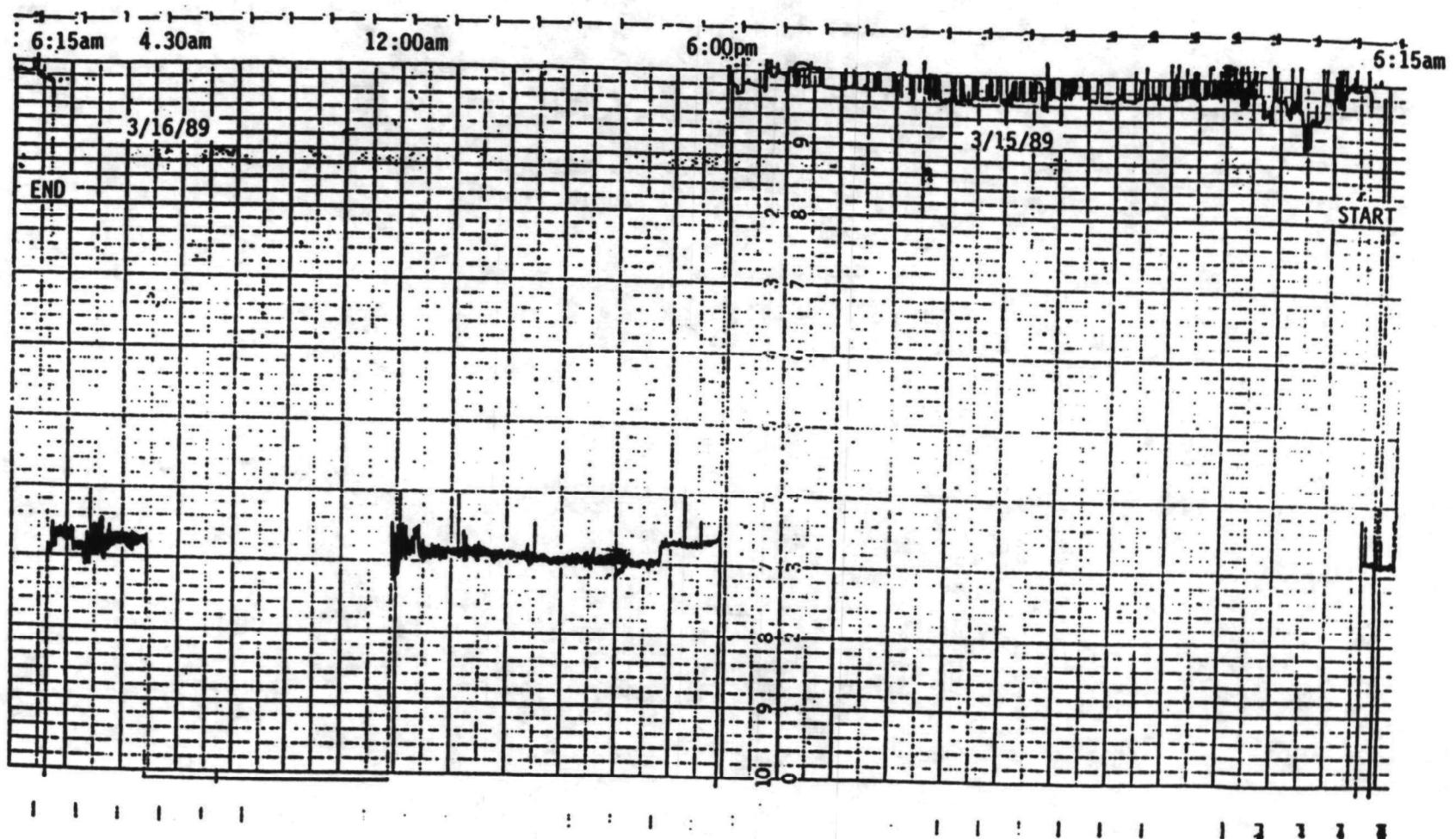
Figure 14. Stability of AM Radio Station at 1.180 MHz. The station operates at full power from 6:15am to 6:00pm. The variation during this operation may be due to unstable transmitter performance.
