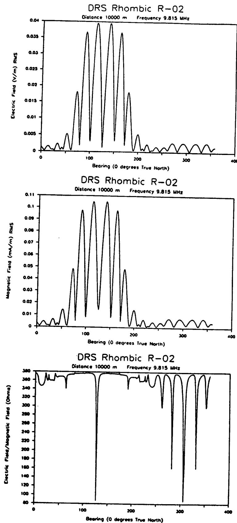
Figure 22. Calculated Fields for Rhombic R-02 at 9.815 MHz
