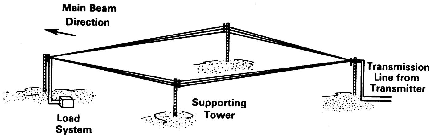
Figure 3. Typical Rhombic Antenna. The antenna is constructed from horizontal wires supported by towers. The main beam is directed about  $10^{\circ}$  above the horizon to reflect off of the ionosphere. For most of the rhombic antennas, the load and transmission line connections can be reversed in order to reverse the direction of the main beam.
