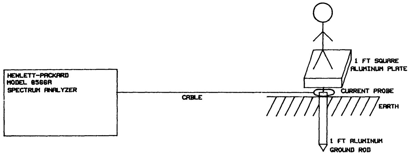
Figure 10. Body Current Measurement System. The current probe is clamped around the ground rod which is in series with ground and the body.
