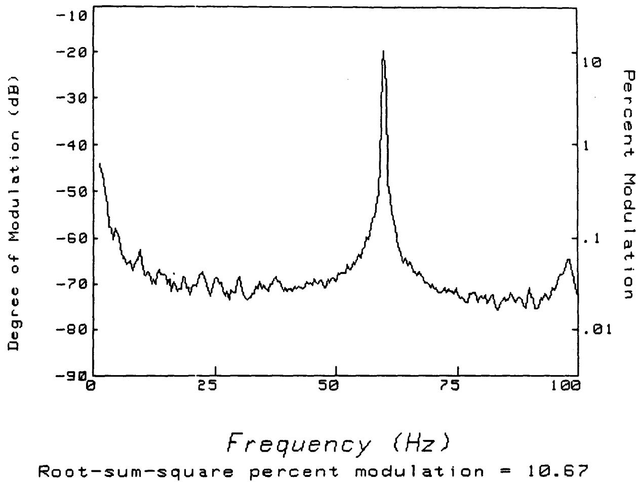
Figure 19. AM Spectrum Analysis of UHF-TV Station.
