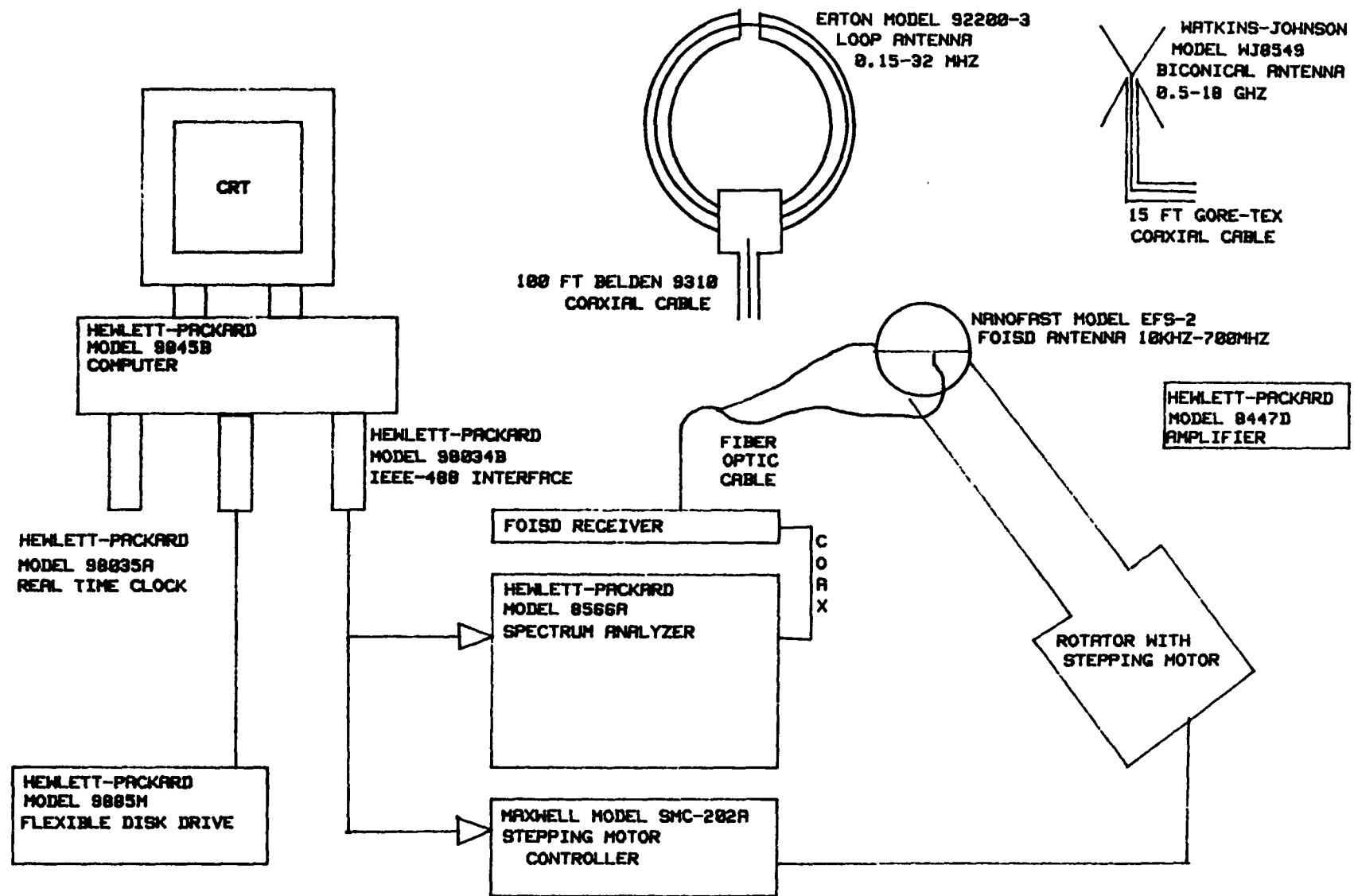
Figure C-1. Automated Field Measurement System. Three different antennas may be connected to the spectrum analyzer. The fiber optically isolated antenna (FOISD) for measuring electric fields at lower frequencies is shown connected. The amplifier can be used to achieve greater sensitivity with the loop and biconical antennas.
