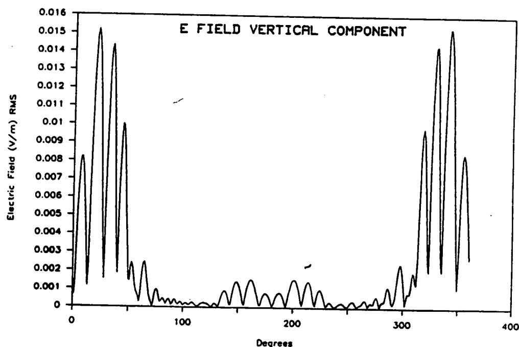
Figure 24. Calculated Electric Field from a Rhombic Antenna in Free Space. Essentially only the vertical component survives the presence of ground.
