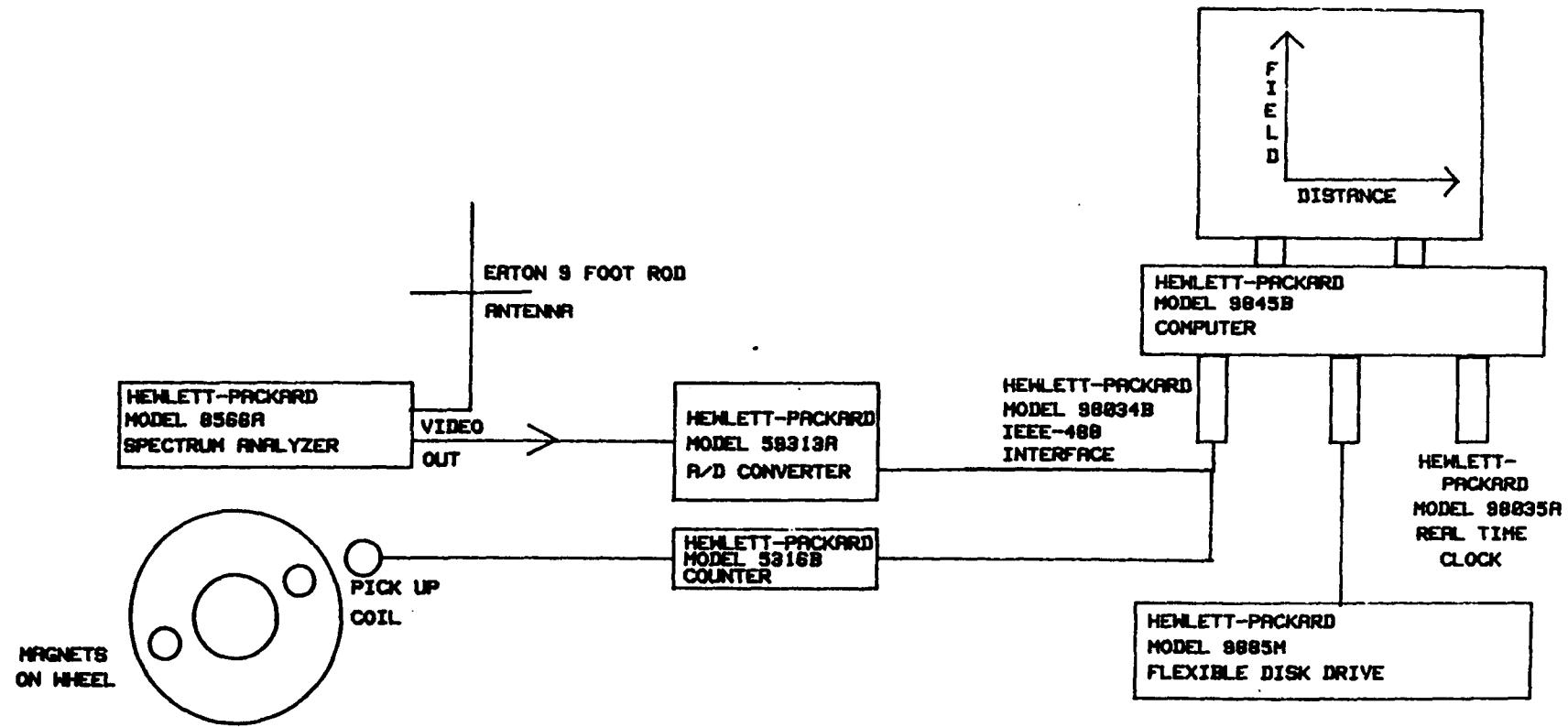
Figure 6. Narrowband Continuous Measurement System. This system allows for measurements at closely spaced intervals of distance.
