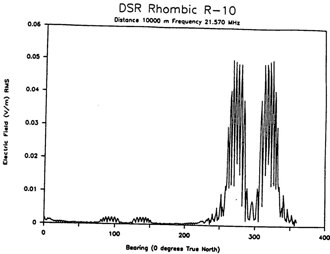
Figure 25. Calculated Electric Field for Rhombic R-10 at 21.57 MHz.
