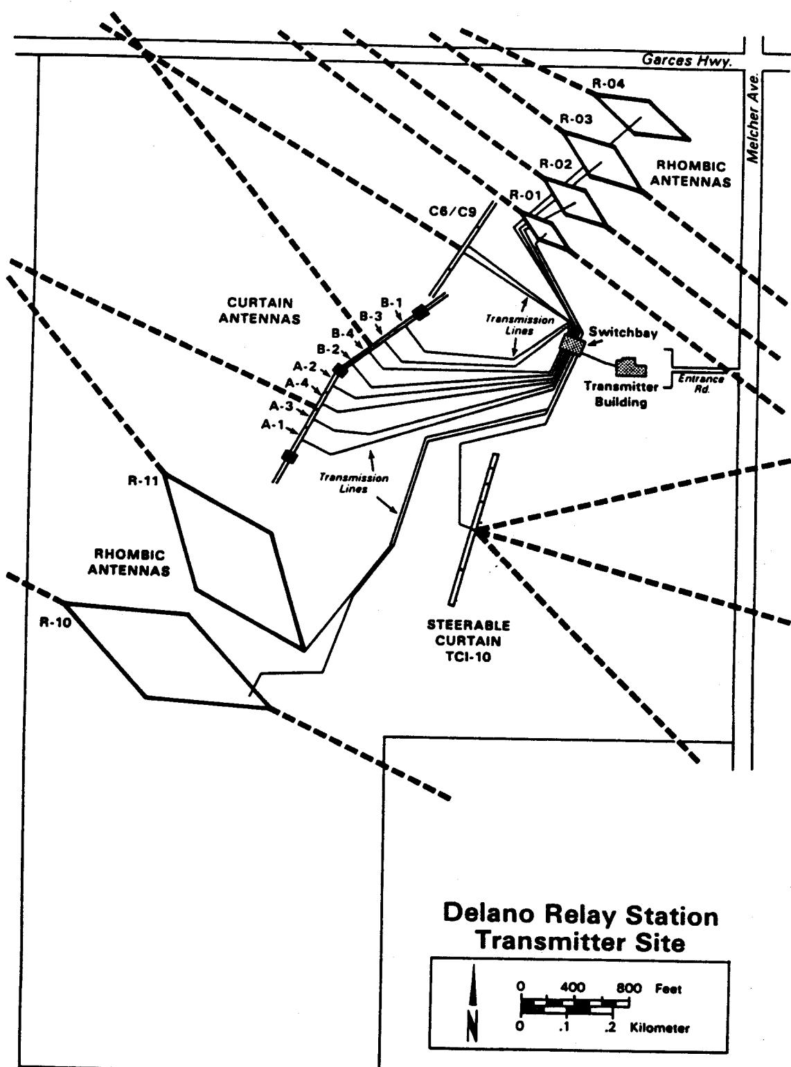
Figure 2. Delano Relay Station. Voice of America site west of Delano. Dashed lines extending from antennas indicate possible directions of propagation.
