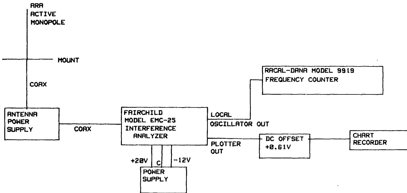
Figure 11. Signal Stability Measurement System. This system can measure the variation over time of RF electric fields for a range of periods of less than one second to days.
