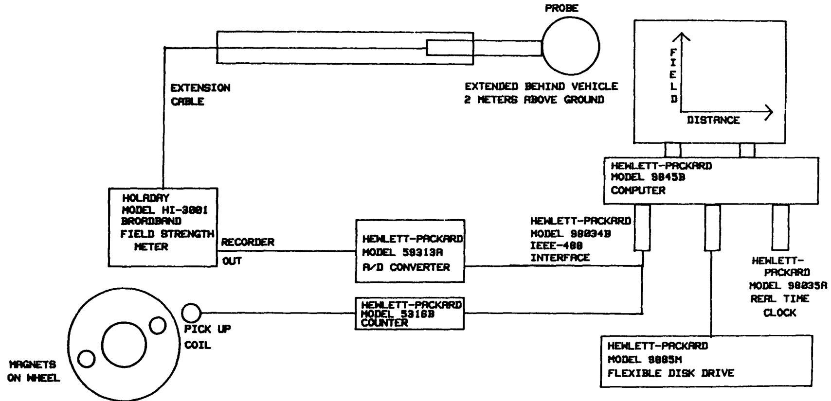
Figure 8. Broadband Continuous Measurement System.
