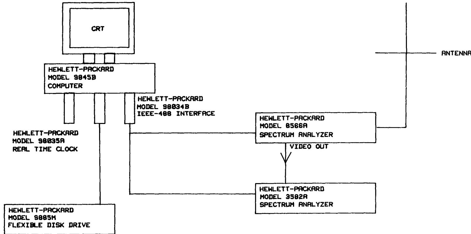
Figure 15. Amplitude Modulation Measurement System. The 8566A Spectrum Analyzer is used as a fixed tuned receiver in linear mode. The video output is proportional to the instantaneous detected RF field strength. Data from the 3582A is used to determine the modulation spectrum.
