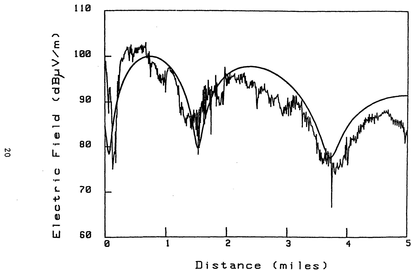
Figure 7. Continuous Measurement Versus NEC Model for Rhombic R-10. Units are in dB with respect to one microvolt per meter. For example  $80 \text{ dB}\mu\text{V}/\text{m} = 0.01 \text{ V}/\text{m}$ . A difference of 20 dB is a difference of a factor of 100 in power density or a factor of 10 in field strength. The smooth curve represents the modeled field strength while the rough line shows the measured field strength.
