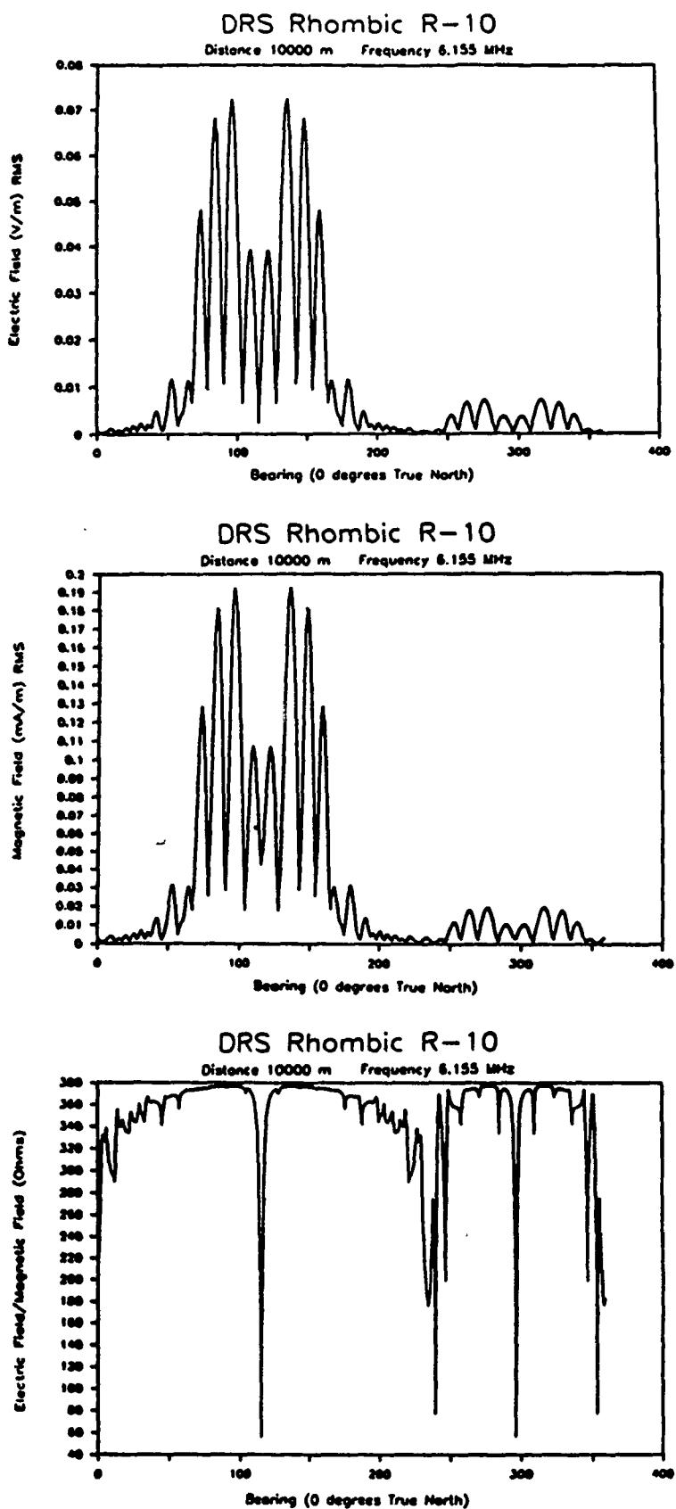
Figure 20. Calculated Fields for Rhombic R-10 at 6.155 MHz.
