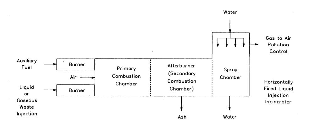
Figure 2-1. Liquid Injection Incinerator
