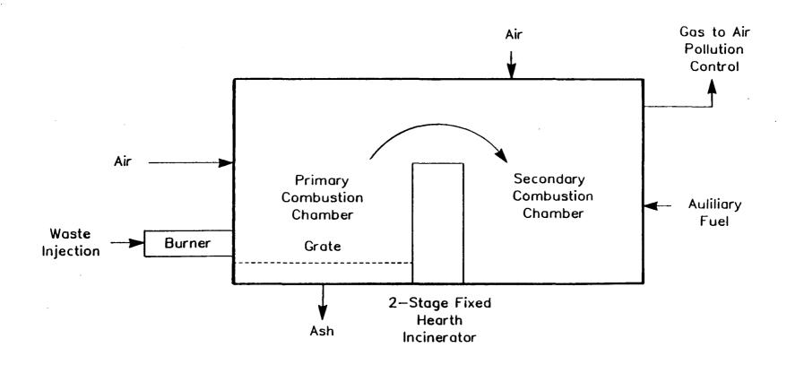
Figure 2-4. Fixed Hearth Incinerator
