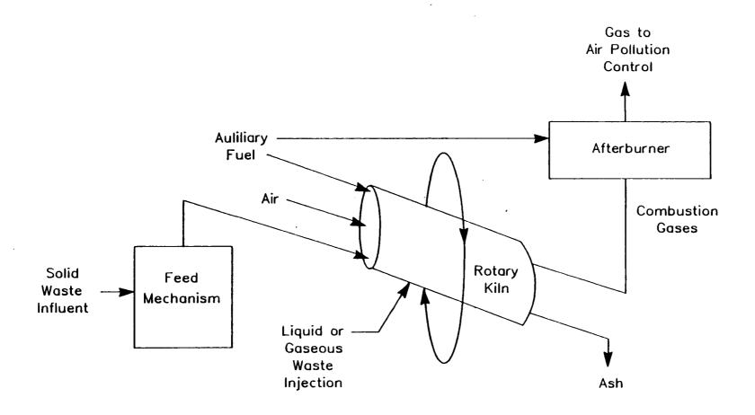
Figure 2-2. Rotary Kiln Incinerator
