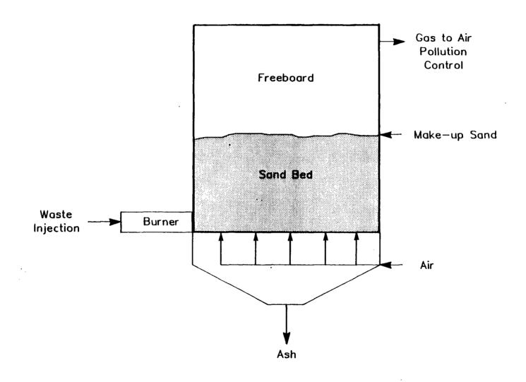
Figure 2-3. Fluidized Bed Incinerator
