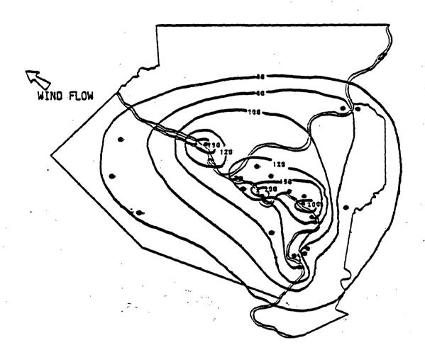
Figure 6. Example of Isopleth Map Showing Pattern of TSP Levels in  $ug/m^3$ . Example is for Southeast Winds.
