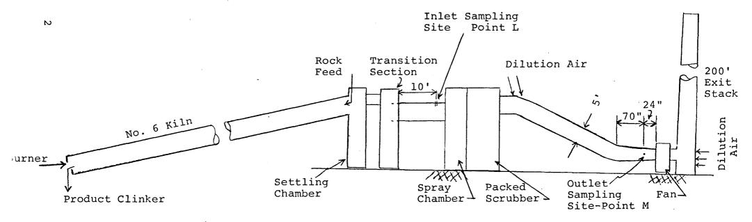
FIGURE 1. DIAGRAM OF ROCK DEFLUORINATION PROCESS AND SAMPLING SITES
