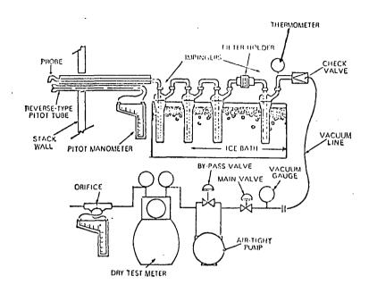
FIGURE 2. SAMPLING TRAIN USED TO DETERMINE FLUORIDE CONCENTRATIONS
