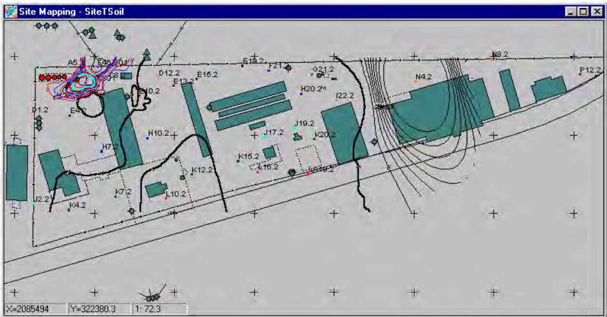
Figure 10. Site T contours for all four chemicals (CTC — black, EDB — blue, DCP — red, and DBCP — light blue ) above their threshold concentrations.
