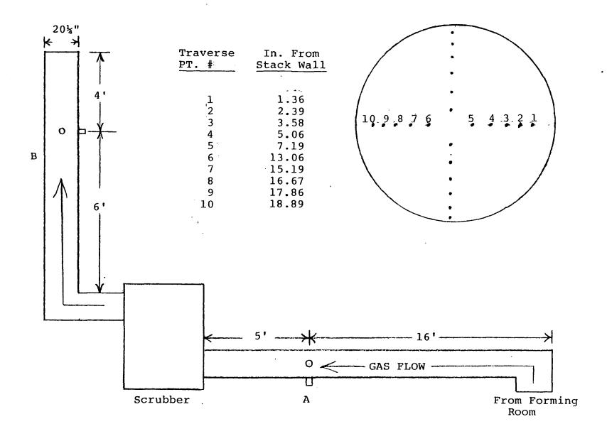
FIGURE 2-1 - H<sub>2</sub>SO<sub>4</sub> SCRUBBER SAMPLING POINTS A & B
