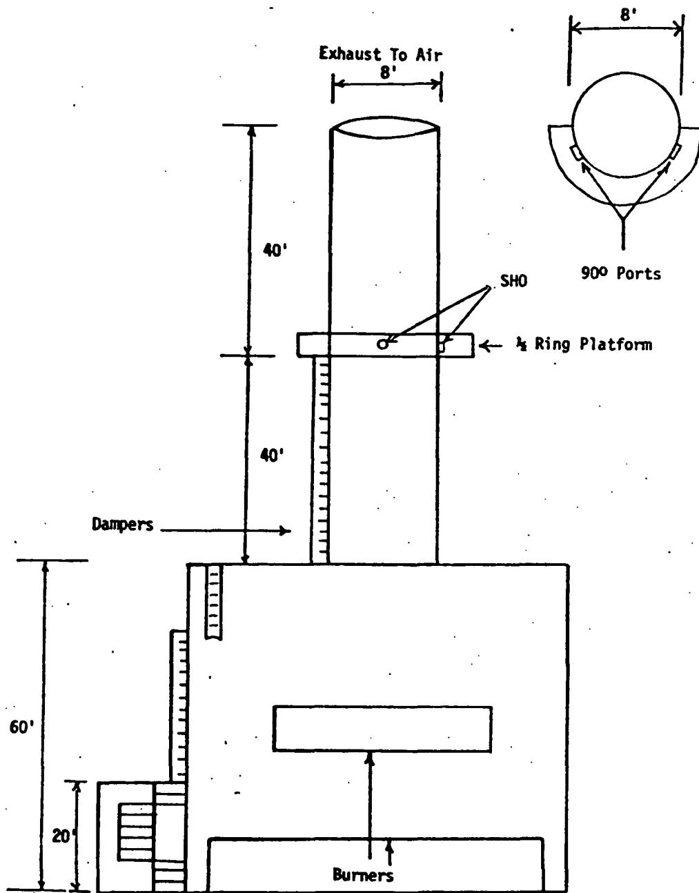
Figure 3-1. Sampling locations steam superheater - Unit 2.
