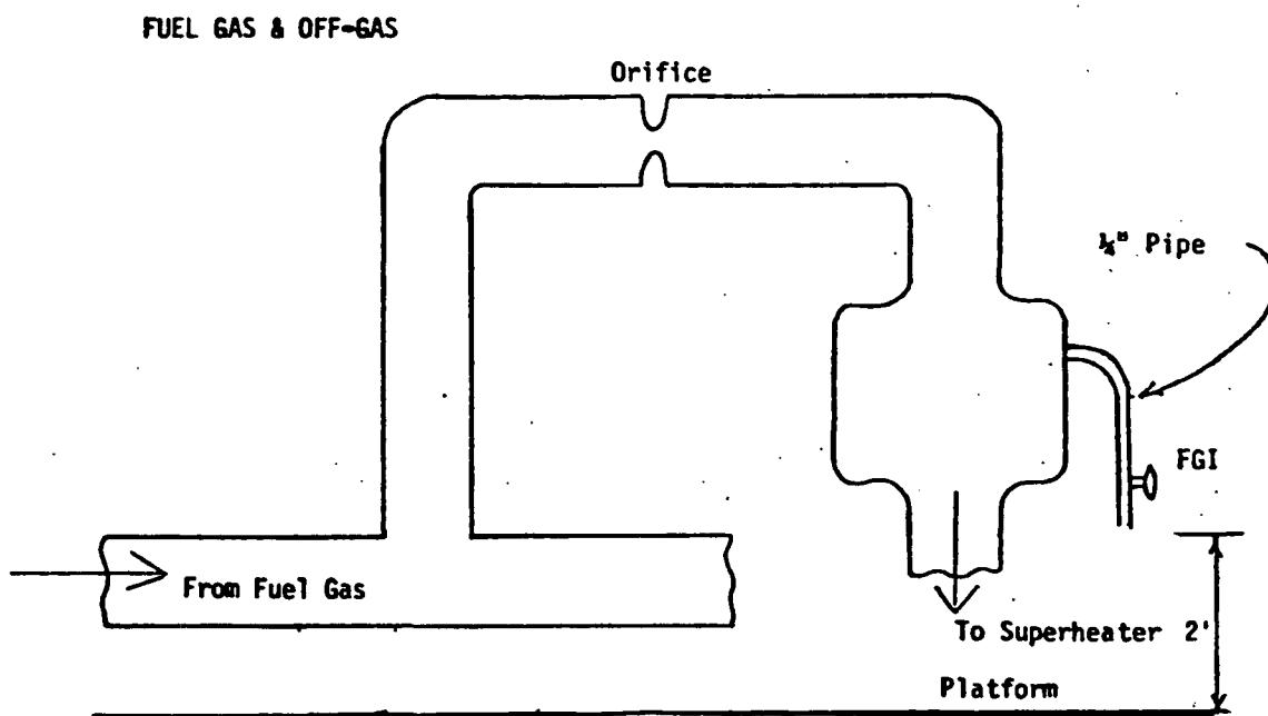
Figure 3-2. Sampling locations off-gas and fuel gas inlets to superheater.
