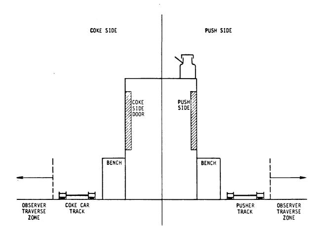
Figure 1. End view of coke oven battery showing recommended traverse zone.
