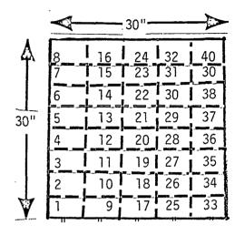
• TRAVERSE POINTS USED FOR THE POST-TEST VELOCITY
