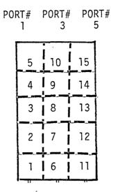
• TRAVERSE POINTS USED FOR TGNMO AND PRELIMINARY VELOCITY TEST.
