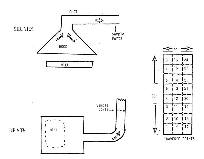
FIGURE 6. SHEET MILL SCHEMATIC
