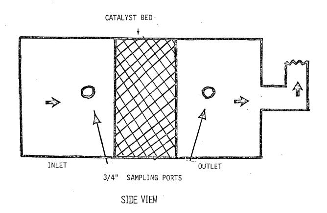
FIGURE 2. CORD COATER OVEN INCINERATOR SCHEMATIC
