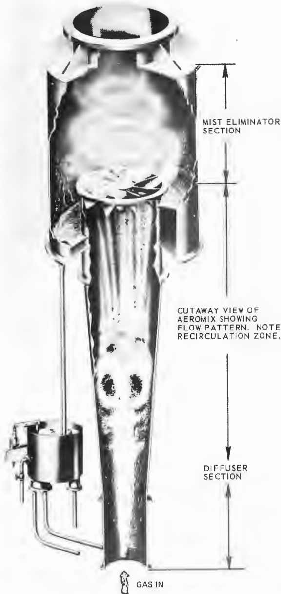
Figure 4-21. Vertical venturi scrubber. (Courtesy of UOP Air Correction Division)
