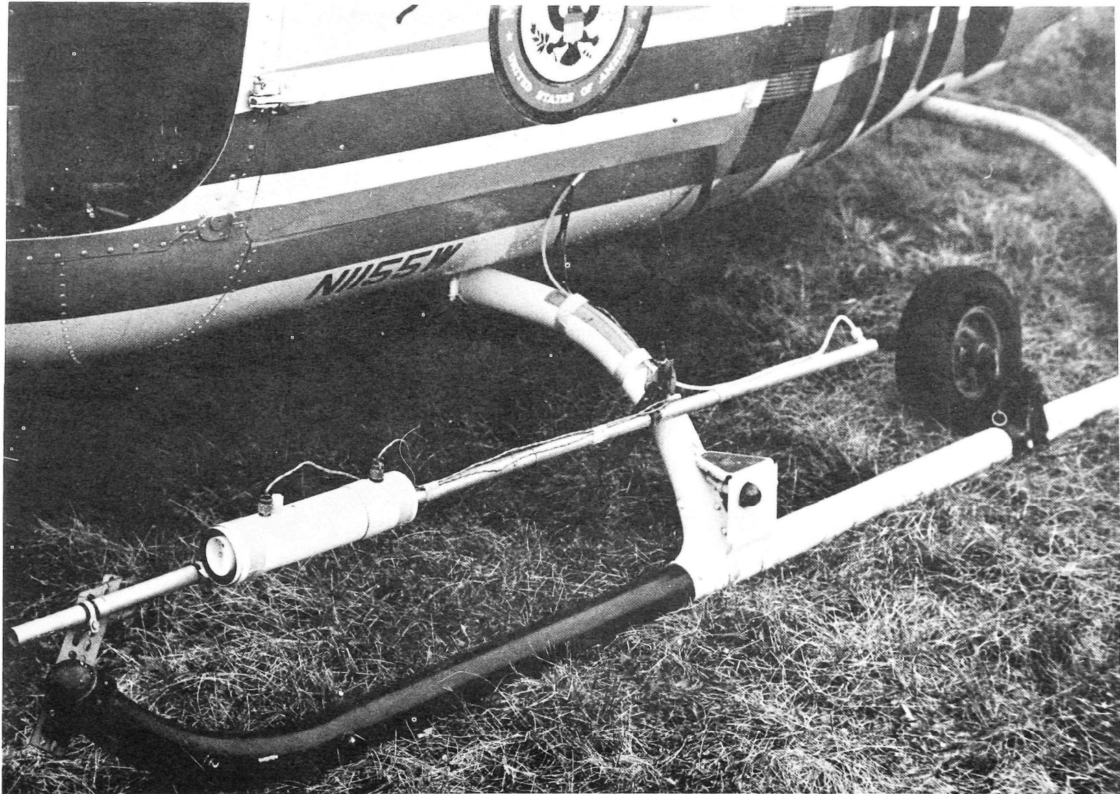
Figure 8. External helicopter probe.
