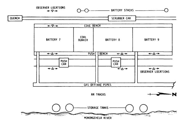
Figure 2. Plan view of Batteries 7, 8, and 9, U.S. Steel Corporation, Clairton, Pennsylvania.
