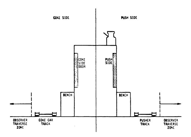
Figure 1. End view of coke oven battery showing recommended traverse zone.
