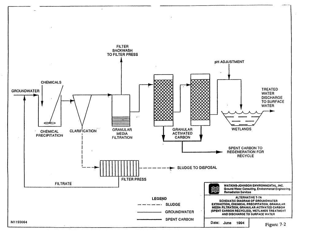
Filtration, Schematic Diagram of Groundwater Extraction, Granular Cart נ (Spail Carbon Recycled), Constructed Wetlands Chemical Precipitation, Granular Media
