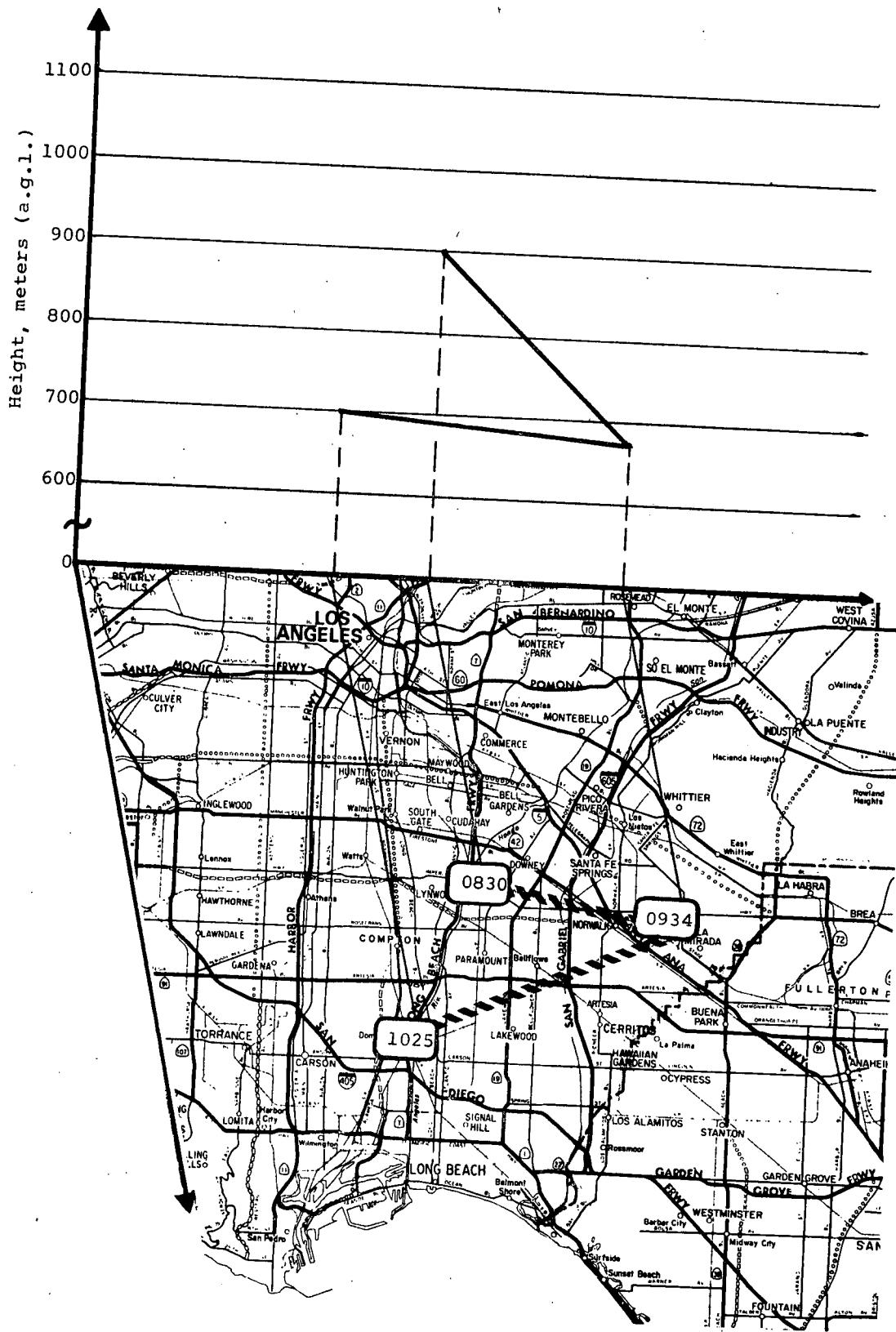
**Figure 35. Mixing layer height along observational route
