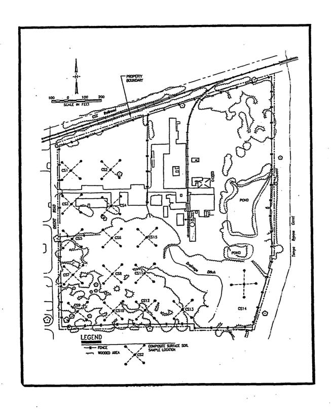
FIGURE 5-2: SOIL BORING LOCATIONS
