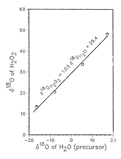
Figure 8. Dependence of  $\delta^{18}O_{\mbox{H}_2O_2}$  on  $\delta^{18}O_{\mbox{H}_2O}$  in a high-voltage discharge process of formation
