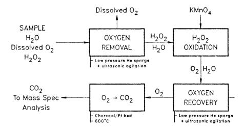
Figure 1. Four-step method for conversion of oxygen in H<sub>2</sub>O<sub>2</sub> (ppb range in water) to CO<sub>2</sub> for mass spectrometric analysis
