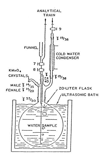
Figure 3. Reaction chamber
