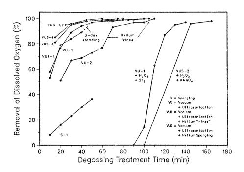
Figure 6. Removal of O<sub>2</sub> from water by various degassing techniques
