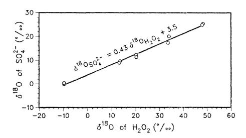
Figure 9. Dependence of  $\delta^{18}{\rm O_{SO_4^{2-}}}$  on  $\delta^{18}{\rm O_{H_2O_2}}$  in oxidation of SO<sub>2</sub> to SO<sub>4</sub><sup>2-</sup>
