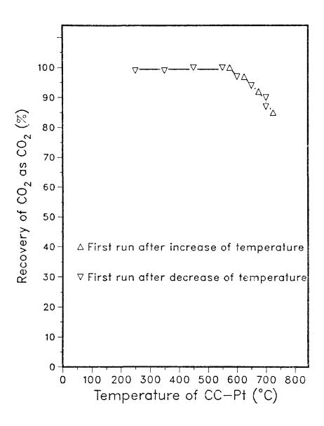
Figure 5. Recovery of CO<sub>2</sub> after exposure to charcoal and platinum at various temperatures
