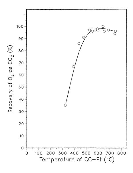
Figure 4. Recovery of O<sub>2</sub> as CO<sub>2</sub> after reaction with charcoal in contact with platinum at various temperatures
