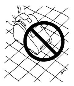
Asbestos has been added to some vinyl floor tiles to strengthen them. Asbestos is also present in the backing on some vinyl sheet flooring. The asbestos is often bound in the tiles and backing with vinyl or some type of binder. Asbestos fibers can be released if the tiles are sanded or seriously damaged, or if the backing on the sheet flooring is dry-scraped or sanded, or if the tiles are severely worn or cut to fit into place.
