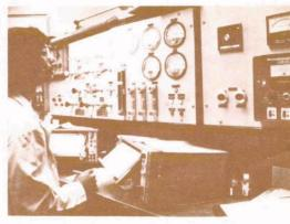
Technician operates an analyzer to determine the amount of pollution in a test vehicle's exhaust.
