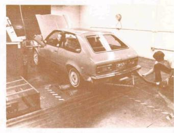
On a dynamometer the driver runs his car through the test cycle of starts, stops and speed changes being displayed on the device beside his window. At right, exhaust fumes are collected for analysis.
