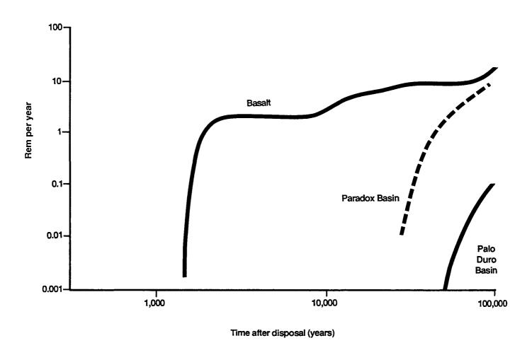
Figure 5-1. Individual doses from ground water use at two kilometers
