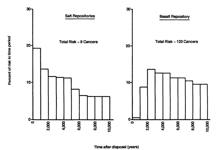
Figure 4-2. Relative incidence of residual risk for model repositories
