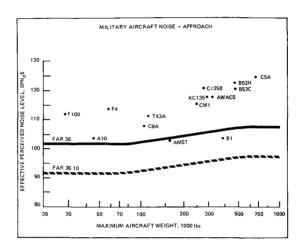
Figure 1. Military Aircraft Noise at Takeoff and Approach as Compared to Federal Aviation Administration's Civil Aircraft Noise Regulations (FAR Part 36)
