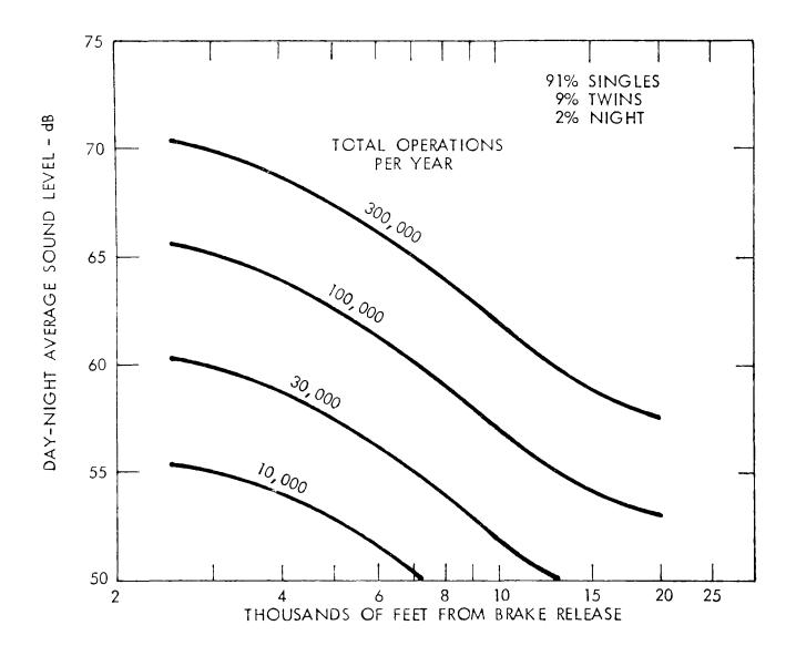
TAKEOFF NOISE FROM PROPELLER - DRIVEN SMALL AIRCRAFT
