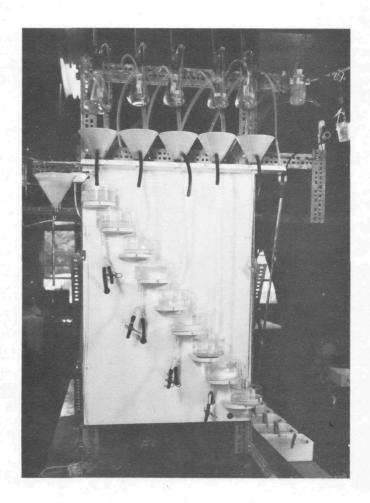
Figure 7. A serial-dilution apparatus designed to deliver 300 ml /min of five concentrations and a control. Several minor changes are used on this diluter.
