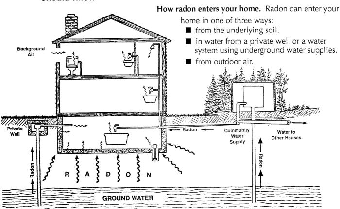
Usually, radon enters a home by seeping through walls and floors from the underlying soil. Radon can seep into a home through dirt floors, cracks in concrete floors and drains, sumps, joints, and tiny cracks or pores in hollow-block walls.
