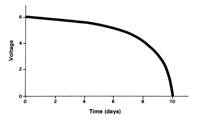
Figure 1. Change of discharge voltage as a function of time for one 40 Ah power supply unit.
