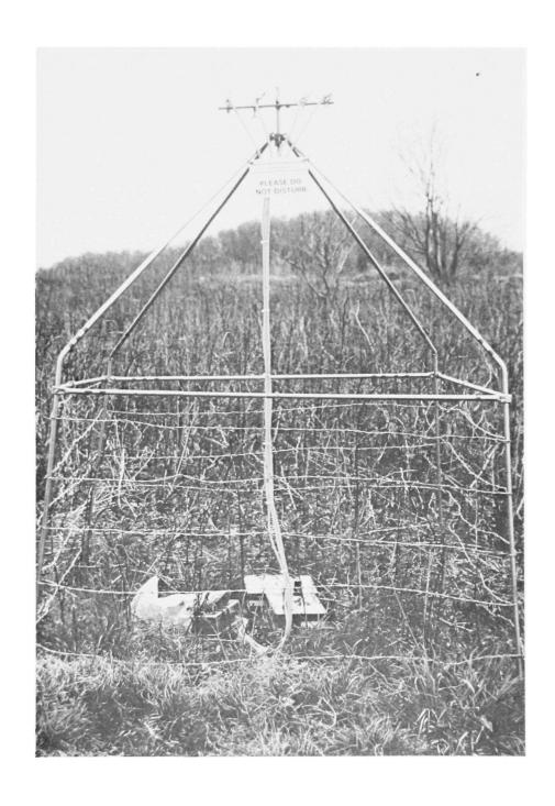
Figure 2. Barbed wire enclosure constructed to prevent people and animals from tampering with air sampling equipment.
